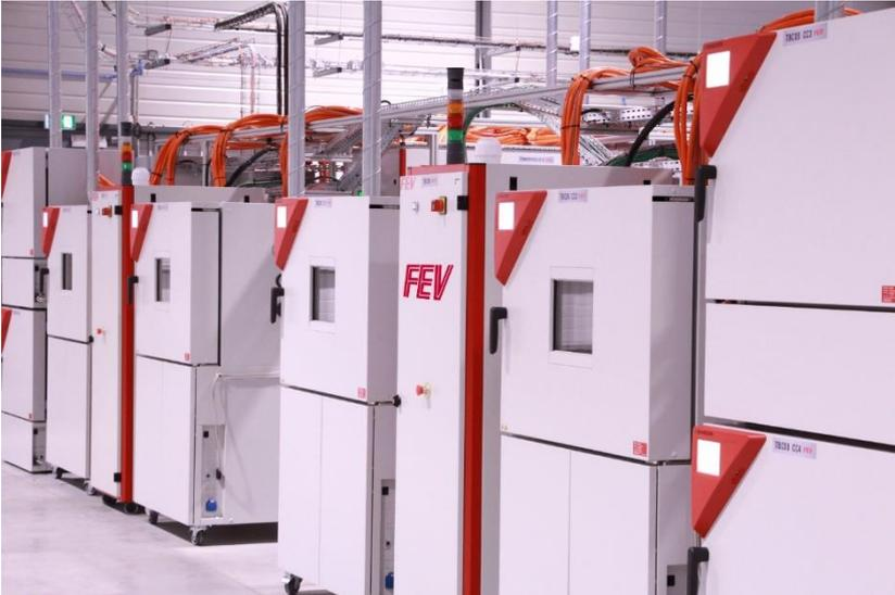
Battery test cells designed by FEV STS: cell testing case – Source: FEV Group
