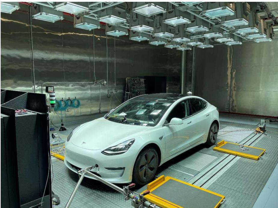
The new solar simulation system plays an important role for globally applicable regulatory tests of both electric vehicles and vehicles with an internal combustion engine.
