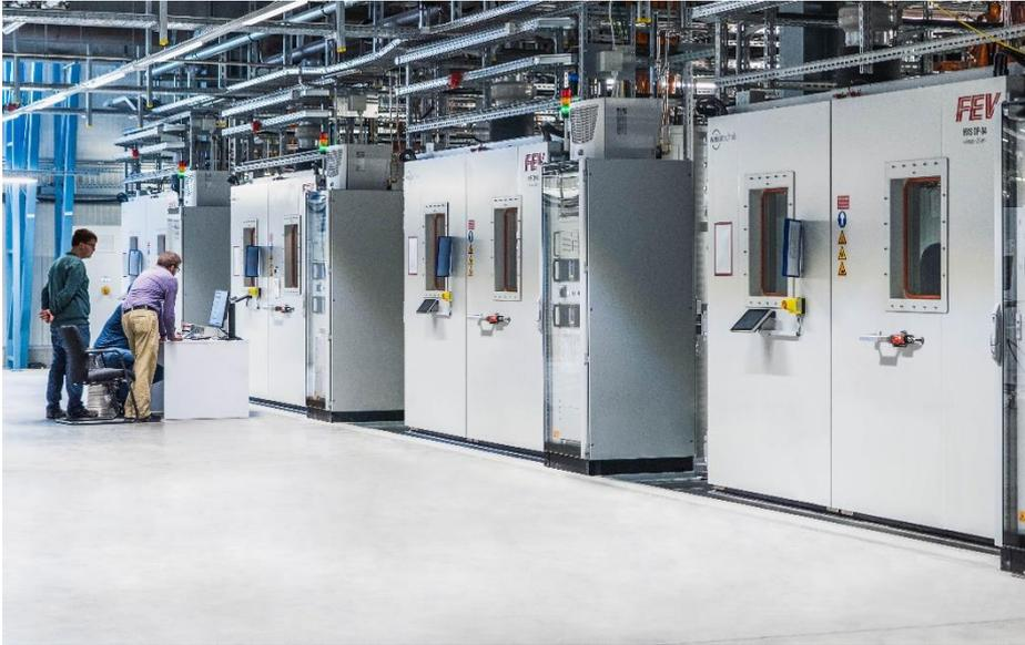
FEV France's new test facility will enable up to two battery packs to be tested at the same time under extreme environmental conditions ranging from -40 to 70 °C.
