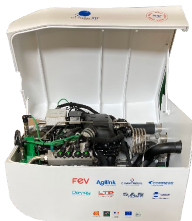
Caption: FEV has developed an hydrogen-fired engine for small aircrafts in a consortium with seven partners
