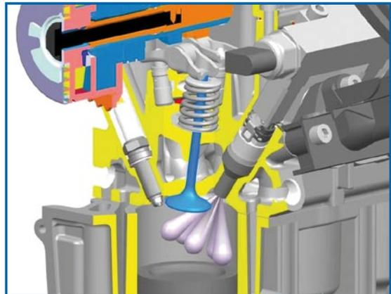
Combustion Chamber with integrated DI Injector
