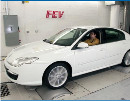
Electric vehicle Renault Laguna of the FEV Hybrid-Testbench during Final Tests
