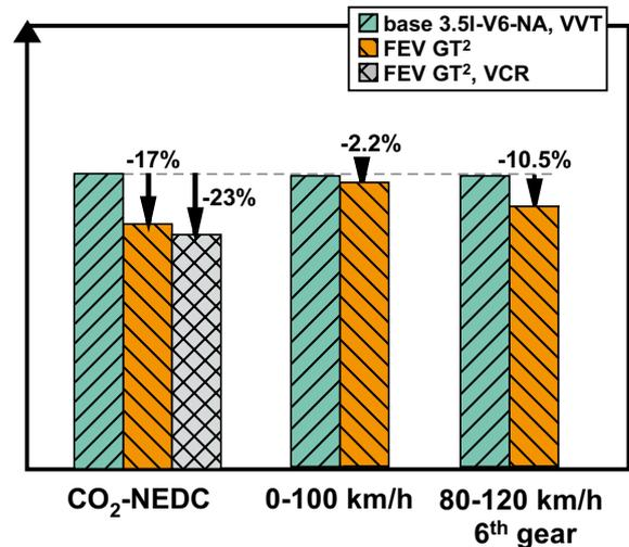
Fig. 8: Comparison of CO<sub>2</sub>-emissions and performance of the GT<sup>2</sup>-concept
