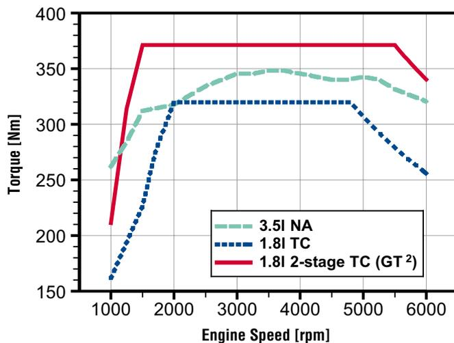
Fig. 7: Full load engine torque curves
