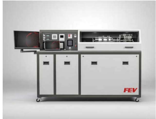
Turbocharger friction loss test bench used to measure the mechanical losses in turbocharger bearings
