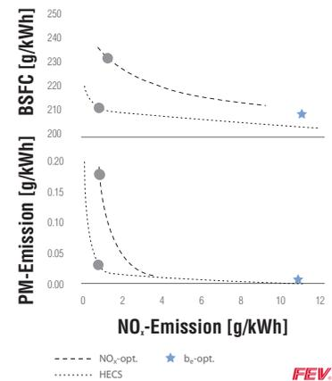
Fig. 1: Emission Performance and Efficiency of the HECS Engine (Part Load Point @ ~2300 rpm)
