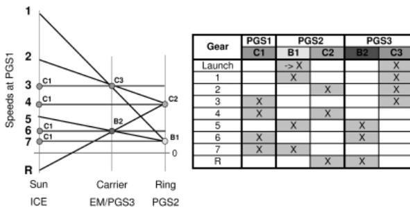
Figure 3: Lever diagram PGS1 and shift element table
