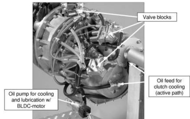
Figure 13: Prototype transmission with external oil pump
