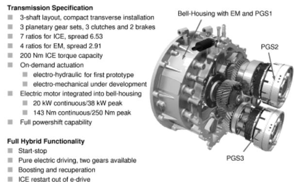
Figure 4: Technical specification of prototype
