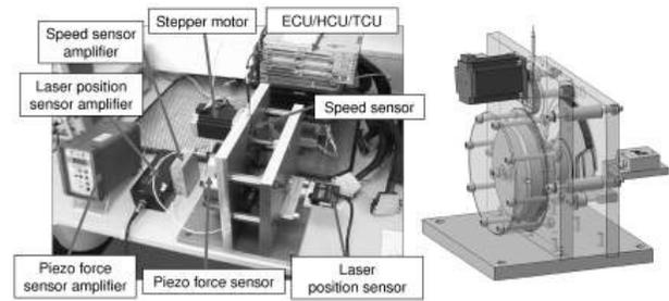
Figure 8: Component test bench
