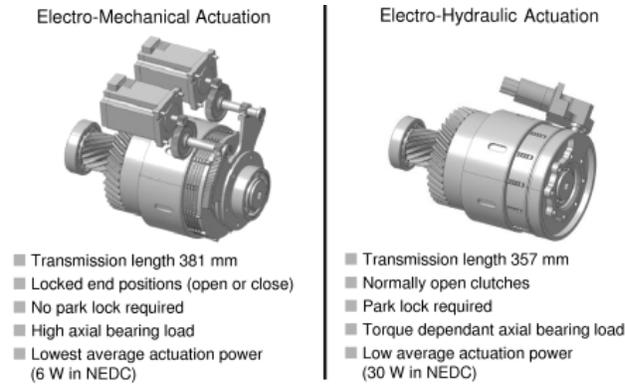
Figure 5: Electro-mechanical and electro-hydraulic actuation systems
