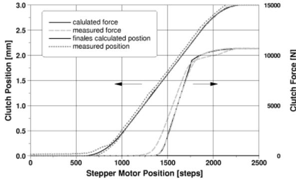
Figure 10: Validation of model based sensor replacement
