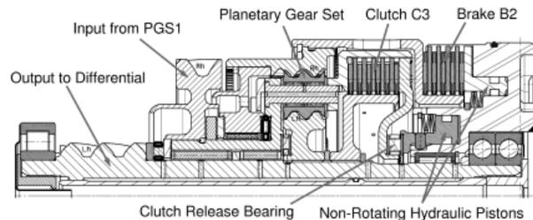
Figure 6: Cross-section of PGS3 with electro-hydraulic actuation
