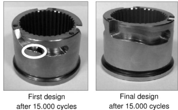
Figure 9: Motion transformer development
