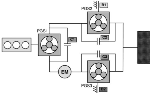
Figure 2: Simplified transmission layout
