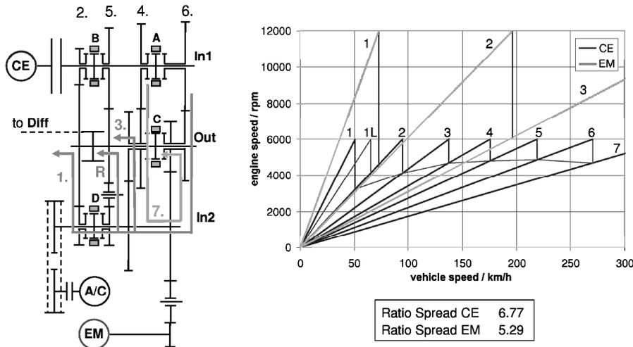
Fig. 1: Gear arrangement and ratio stepping of 7H-AMT
