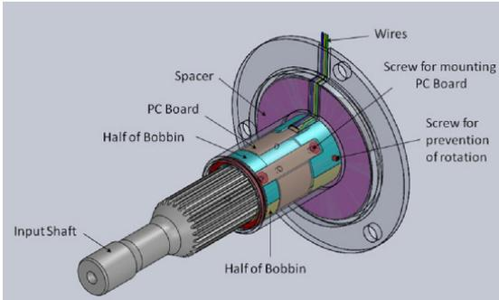
Fig. 6: Torque sensor integration
