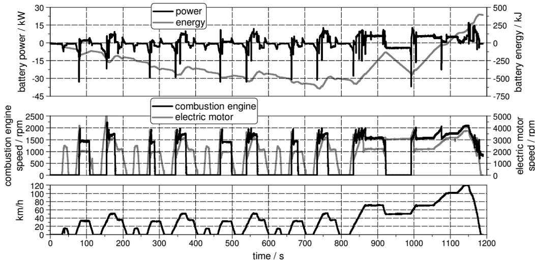
Fig. 5: 7H-AMT demonstrator vehicle in NEDC cy
