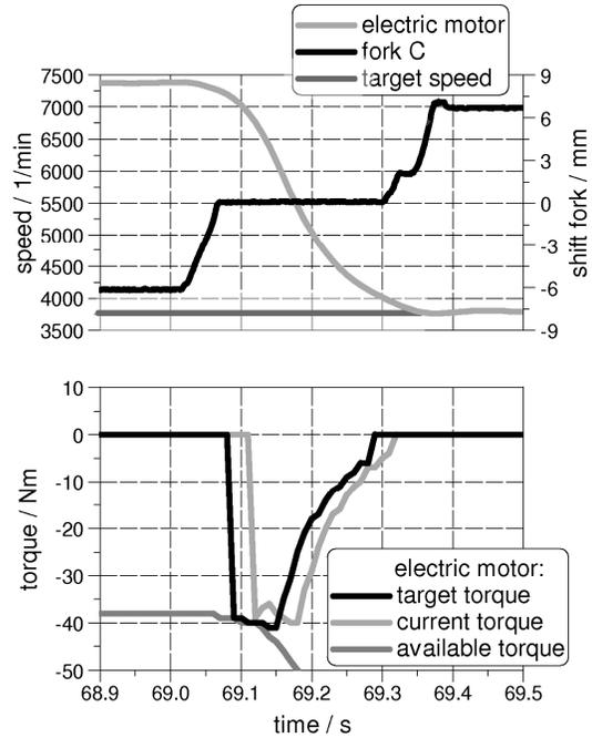
Fig. 3: Electric motor shift with 7H-AMT
