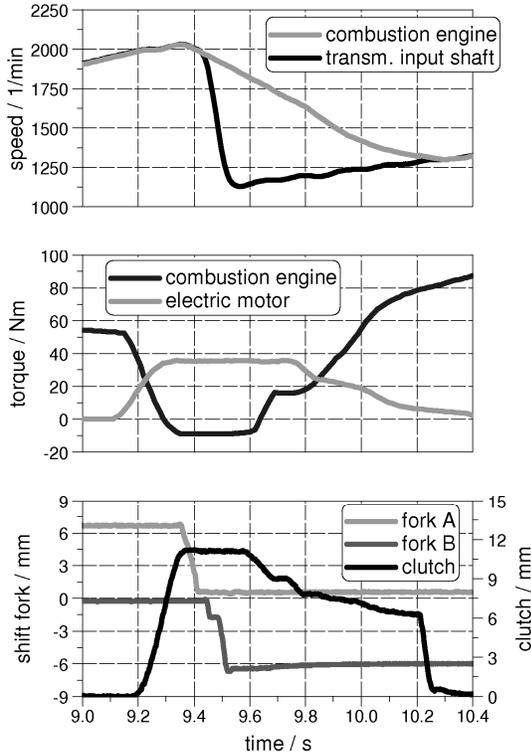
Fig. 2: Combustion engine shift with 7H-AMT
