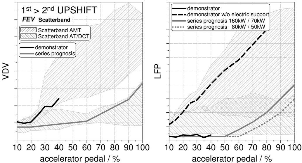
Fig. 4: Shift quality of combustion engine shifts in FEV scatterband.
