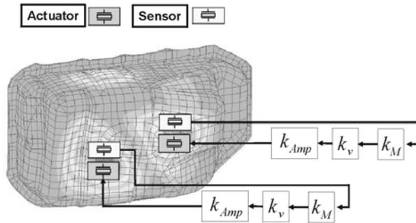
Figure 9: Block Diagram of the Collocated Controller
