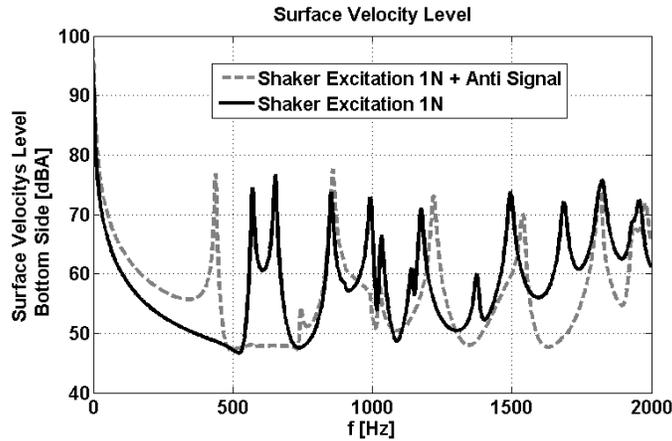
Figure 4: Surface Velocity with and without Anti-signal
