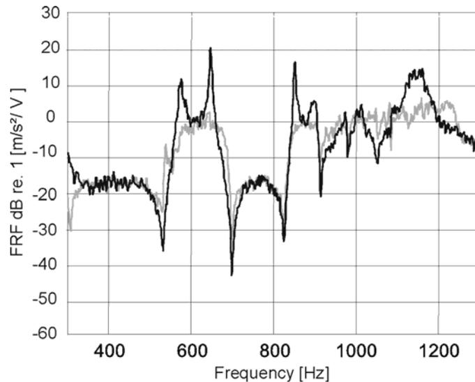
**Figure 14: Frequency Response Function of Shaker Input Signal to Acceleration at Patch 1 Position without Adaptive Feedback Control – Black Curve and with Adaptive Feedback Control – Gray Curve**
