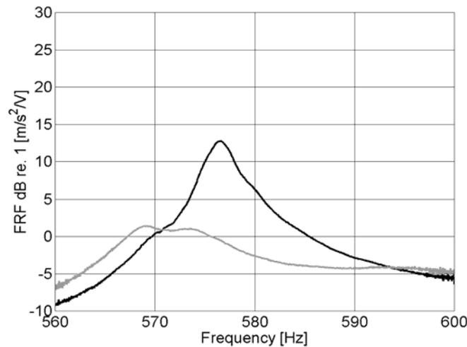
Figure 12: Frequency Response Function of Shaker Input Signal to Acceleration at Patch 1 Position without Semi-passive Damping – Black Curve and with Semi-passive Damping (R=100 Ohm) – Gray Curve
