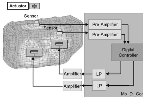
Figure 10: Block Diagram of the Adaptive Feedback Controller
