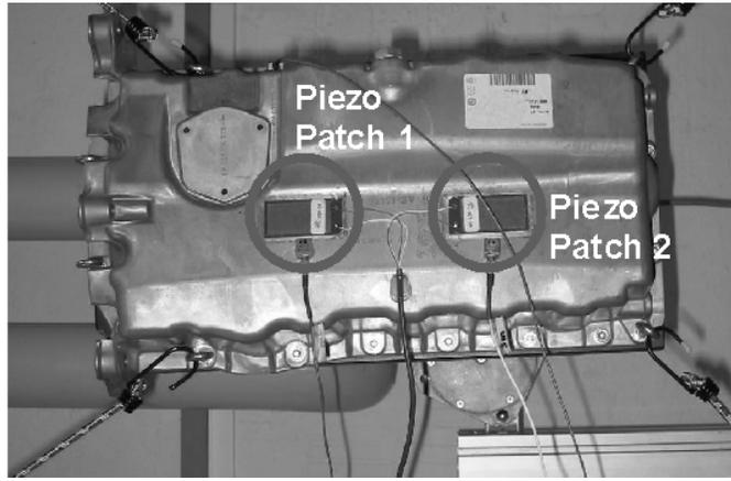
Figure 5: Oil Pan Test Setup with Two Piezo Patches
