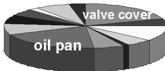
Figure 1: Sound Power Share of a Passenger Car Powertrain
