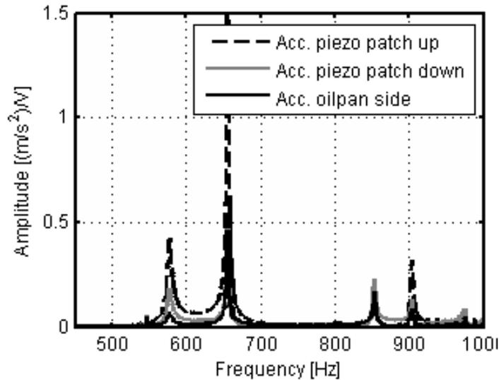
Figure 6: Frequency Response Function of Shaker Excitation to Acceleration Signal for Different Sensor Positions
