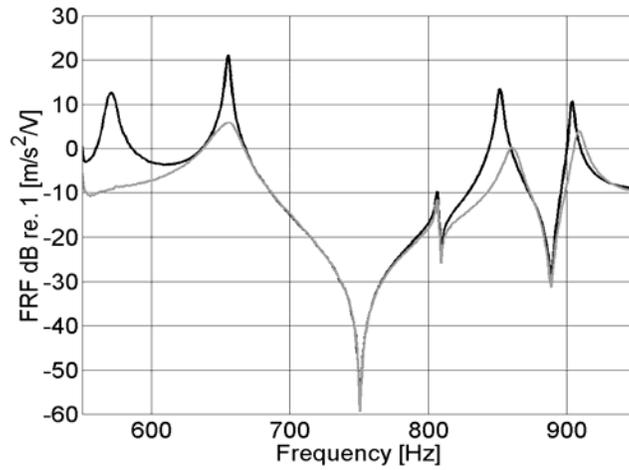
**Figure 13: Frequency Response Function of Shaker Input Signal to Acceleration at Patch 1 Position without Control – Black Curve and with Collocated Control – Gray Curve**
