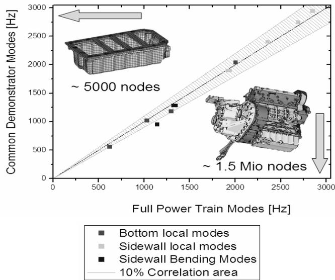
Figure 2: Common Oil Pan Demonstrator Derived from Full Powertrain
