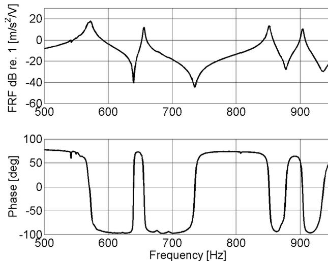
Figure 8: Frequency Response Function between Driving Signal of Patch 1 to Acceleration at Sensor 1
