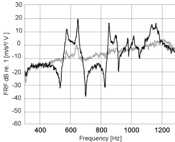
Figure 15: Frequency Response Function of Shaker Input Signal to Acceleration at Patch 1 Position without Adaptive Feedforward Control – Black Curve and with Adaptive Feedforward Control – Gray Curve
