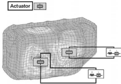
Figure 7: Block Diagram of the Semi-passive Damping System
