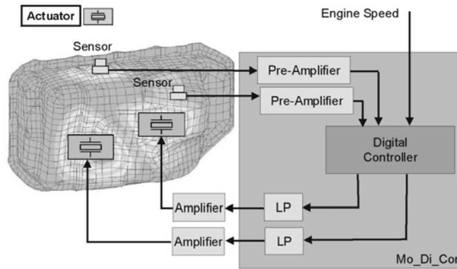
Figure 11: Block Diagram of the Adaptive Feedforward Controller
