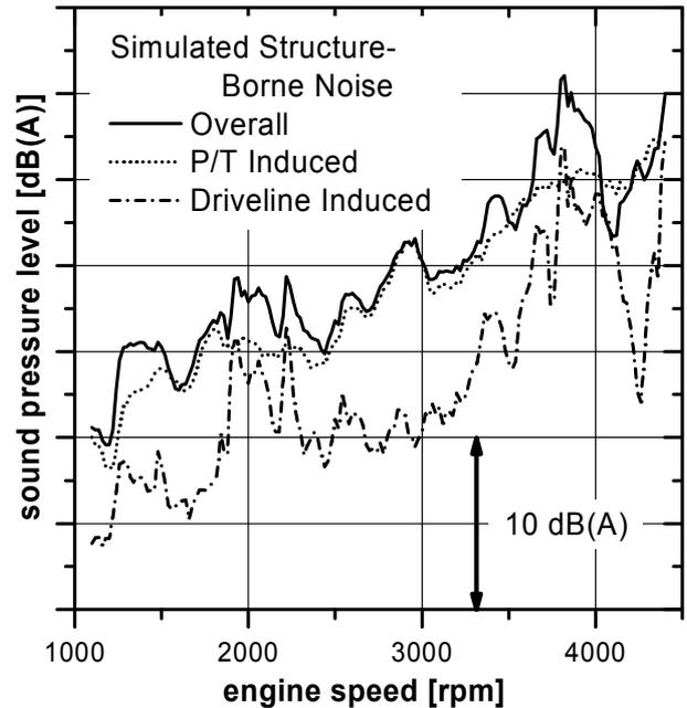
**Fig. 13 Decomposition of simulated structure-borne noise level into powertrain induced and driveline induced noise**
