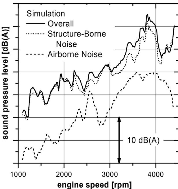
Fig. 6: Decomposition of interior noise level into airborne and structure-borne share (full load)
