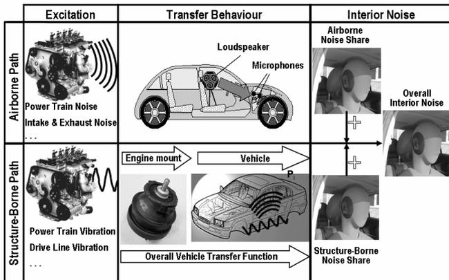
**Fig. 3: Procedure of Vehicle Interior Noise Simulation (VINS)**
