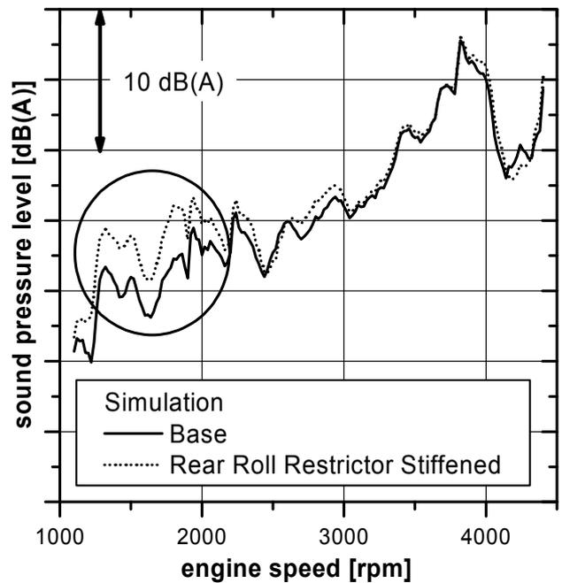
Fig. 11: Simulated overall noise level of base variant v/s modified mounting system with stiffer rear roll restrictor
