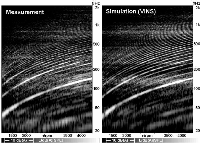
Fig. 5: Campbell diagram of direct measured v/s simulated vehicle interior noise (full load)
