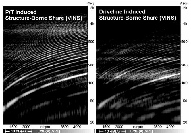
**Fig. 14 Frequency content of simulated powertrain induced and driveline induced structure-borne noise shares**
