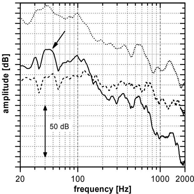
Fig. 9: Transfer functions of the rear roll restrictor, vertical direction
