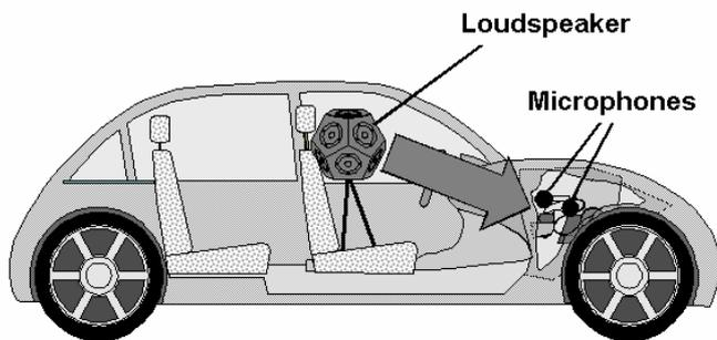
**Fig. 1: Reciprocal measurement of airborne noise transfer functions**
