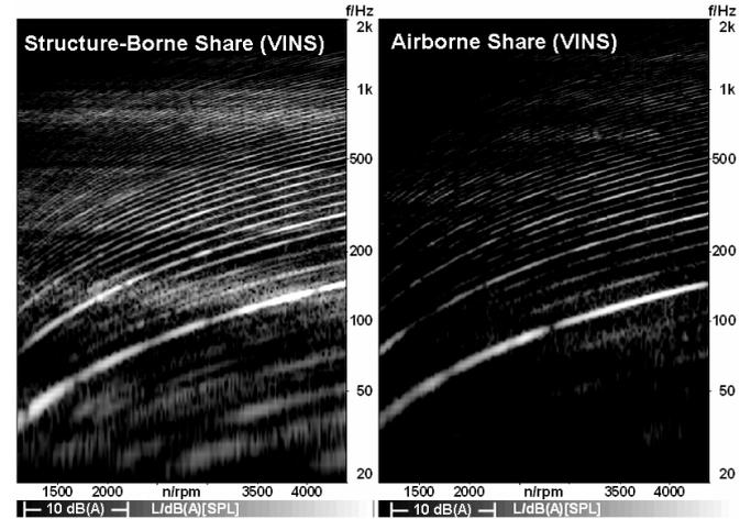
Fig. 7: Spectral content of airborne and structure-borne share of interior noise (full load)
