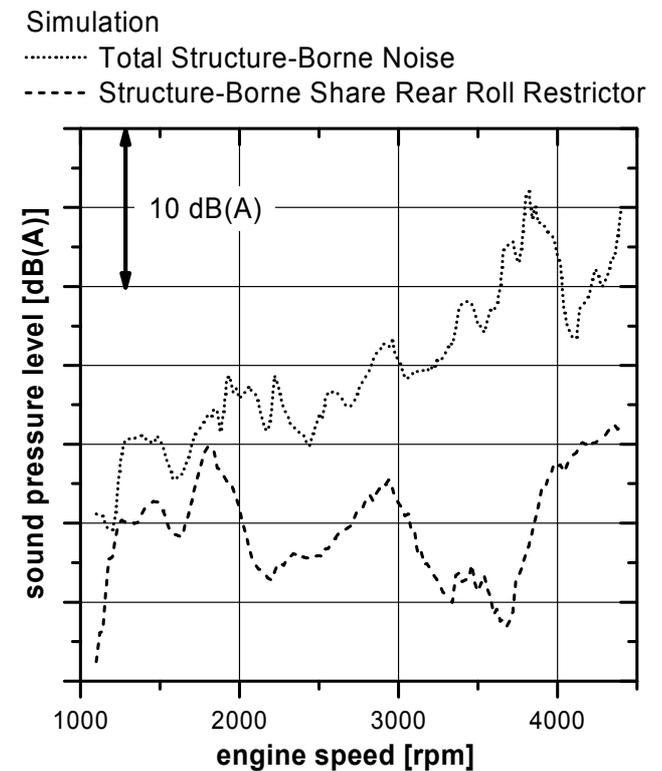
Fig. 8: Comparison of simulated structure-borne noise and the noise share from the rear roll restrictor (full load)
