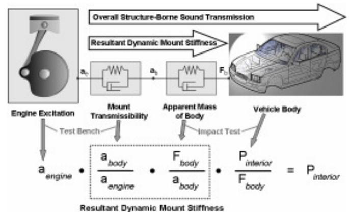
**Fig. 2: Measurement and calculation of dynamic mount stiffness and overall structure-borne transfer function**
