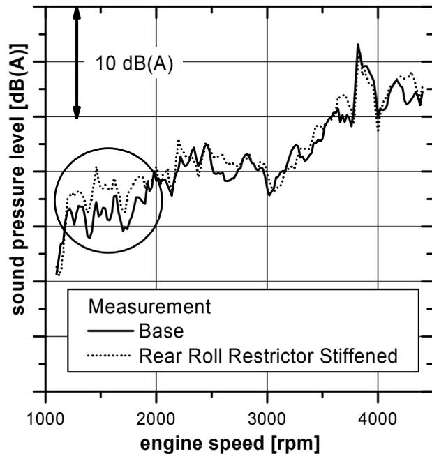
**Fig. 12: Measured overall noise level of base variant v/s modified mounting system with stiffer rear roll restrictor**
