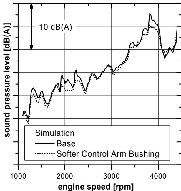
**Fig. 15: Simulated effect of reduced control arm bushing stiffness on interior noise**
