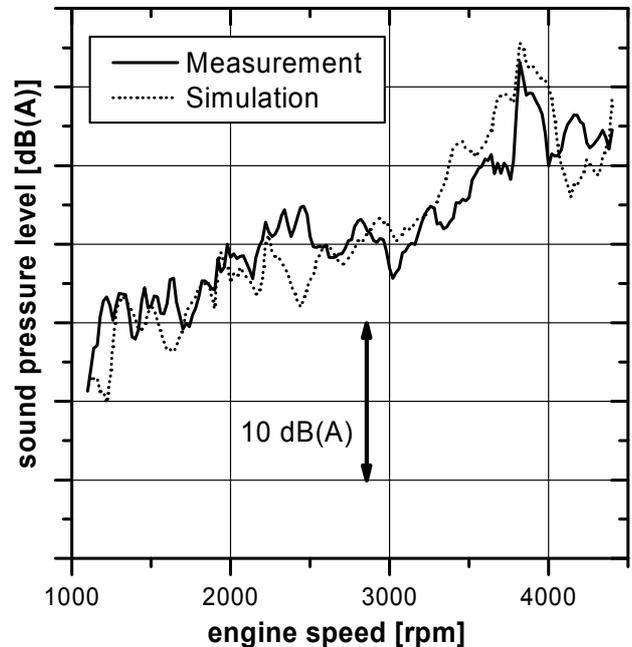
**Fig. 4: Interior noise level of direct measured v/s simulated vehicle interior noise (full load)**
