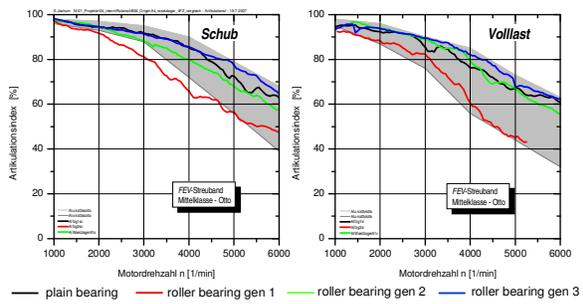
**Figure 7:** Articulation index, artificial head at passenger seat, coasting (left) and full load (right), 2nd gear
