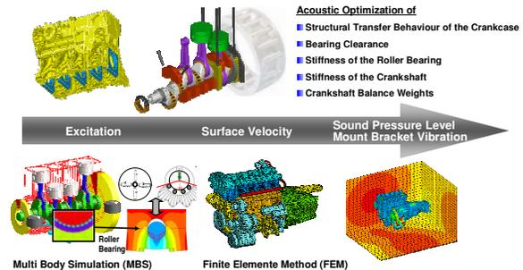
Figure 1: CAE-supported development and optimization procedure of a roller bearing engine by MBS, FEM and BEM calculation
