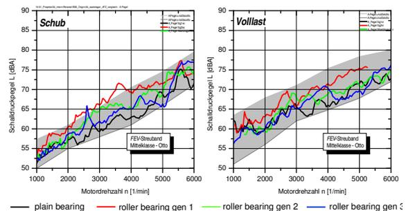
**Figure 5:** A-weighted level, artificial head at passenger seat, coasting (left) and full load (right), 2nd gear.
