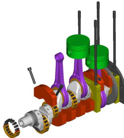
**Figure 3:** Crank train design of roller bearing engine generation 3.
