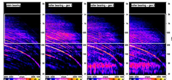
**Figure 4:** A-weighted campbell diagram, artificial head at passenger seat, coasting, 2nd gear
