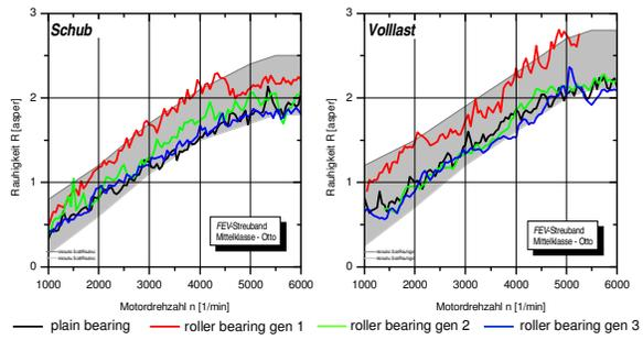
**Figure 6:** Roughness, artificial head at passenger seat, coasting (left) and full load (right), 2nd gear.
