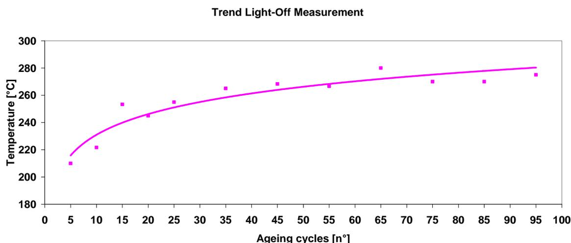
Fig. 13: Light-off upon aging of a DOC measured on hot gas aging test bench
