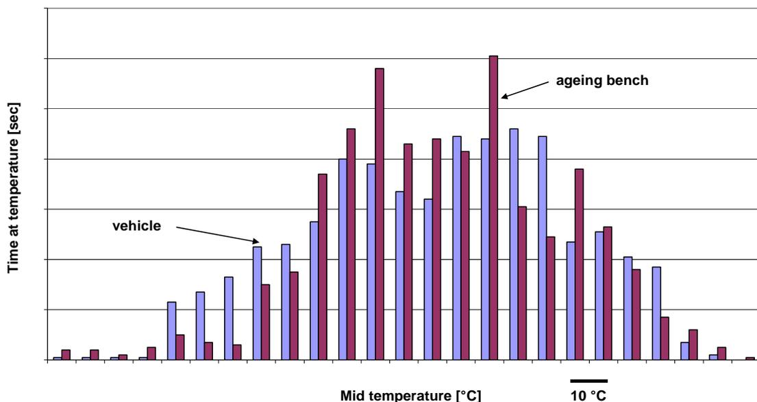
Fig. 12: Exhaust temperature histogram of the engine and hot gas test stand aging profile
