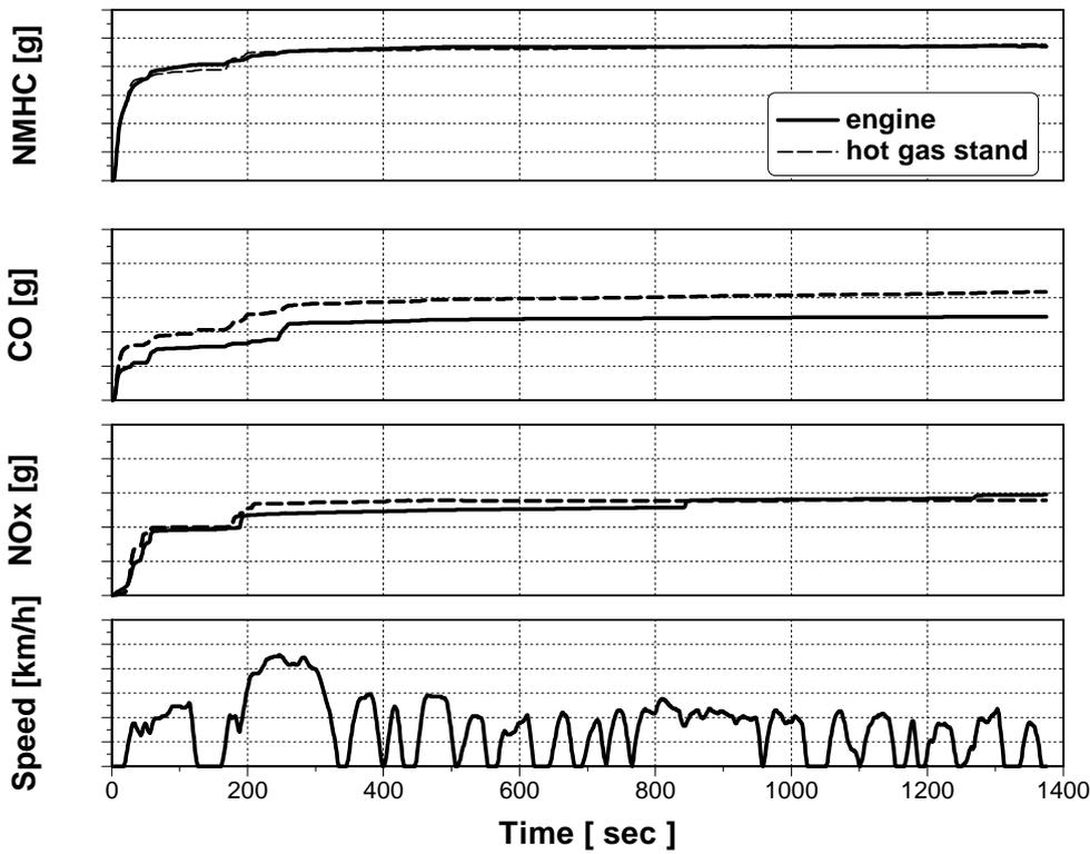
Fig. 10: FTP emission comparison with different aging methods
