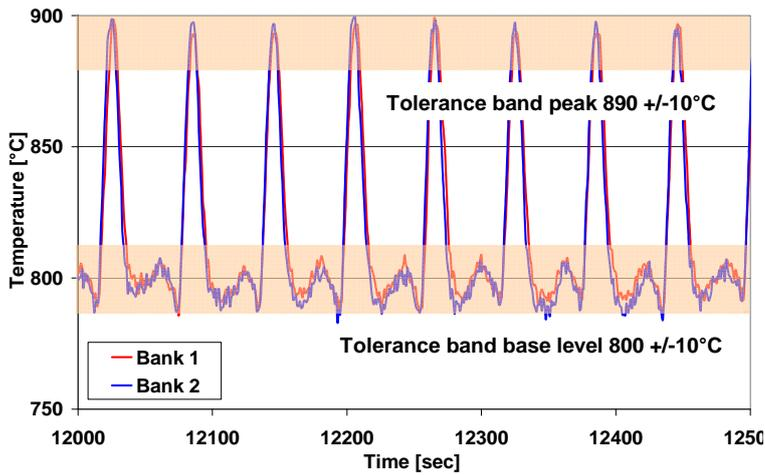
Fig. 6: Standard bench cycle run on aging test bench
