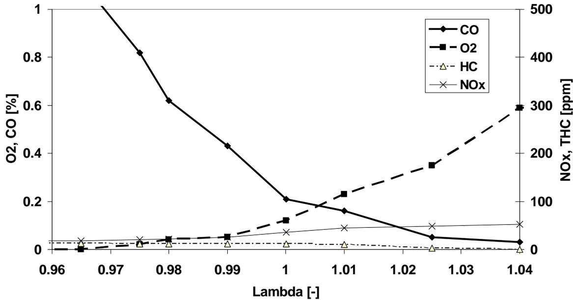
Fig. 5: Burner exhaust emission at 60 gram / sec, 800°C
