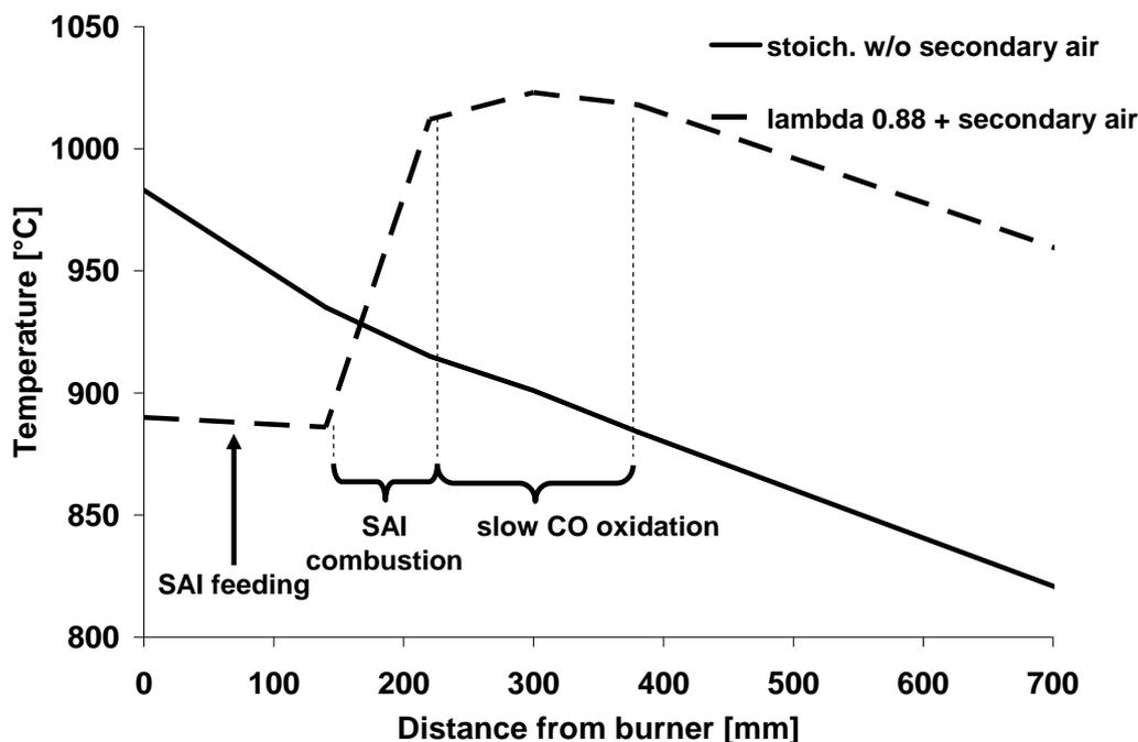
Fig. 15: Secondary air reaction / main and delayed oxidation used for configuration B
