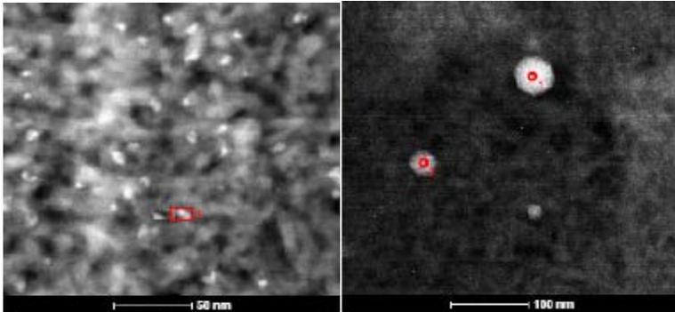
Fig. 1: Comparison of vehicle fresh (left) and aged (right) washcoat active center diameter and distribution
