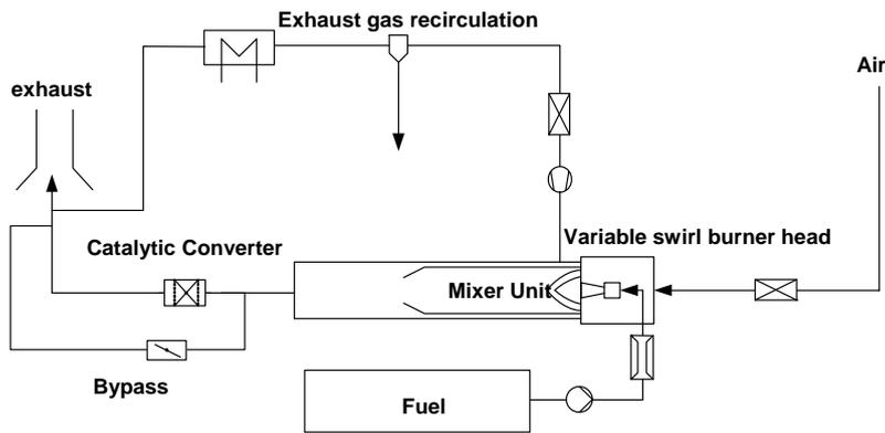
Fig. 2: Hot gas aging test bench schematic
