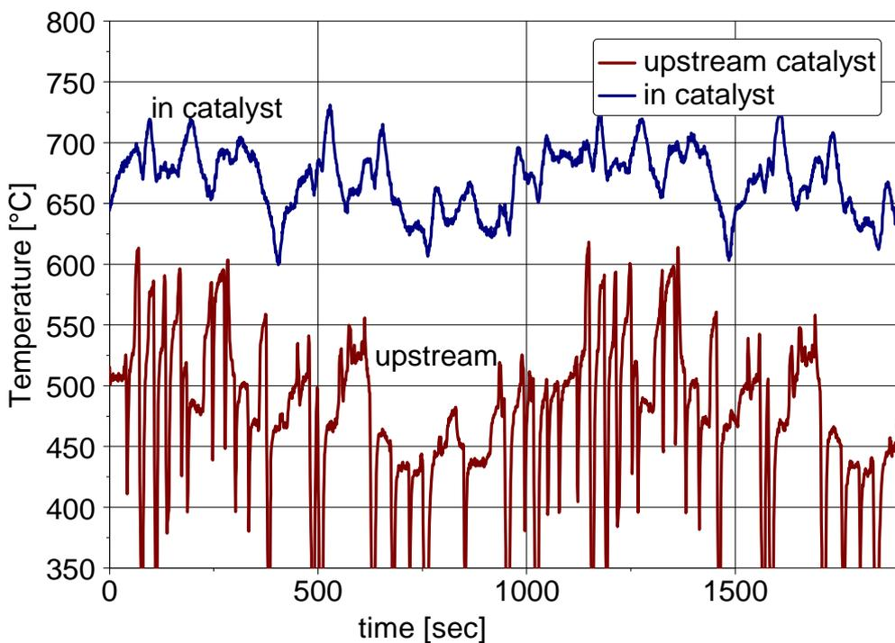
Fig. 11: Dynamic simulation of the drive cycle on the hot gas test stand
