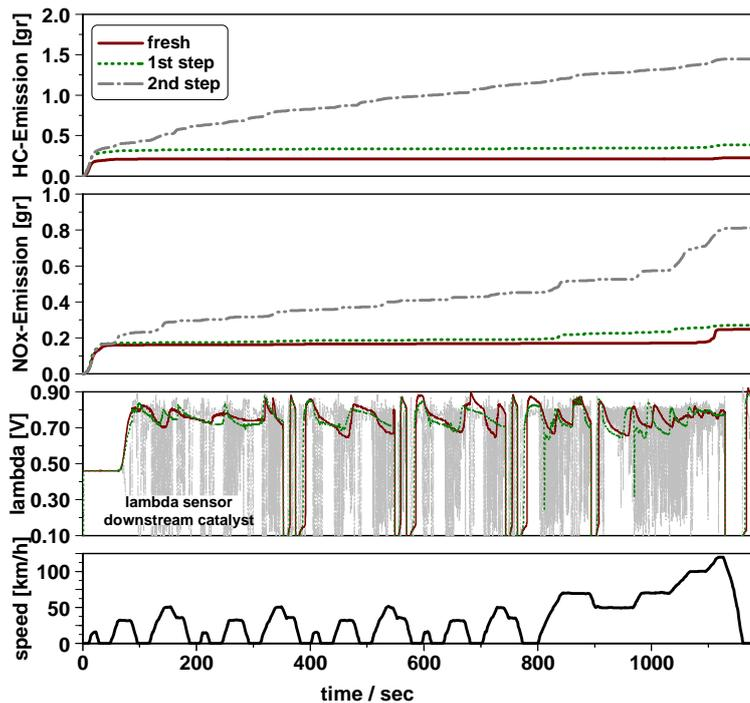
Fig. 17: NEDC emission with catalyst aged using method (B)
