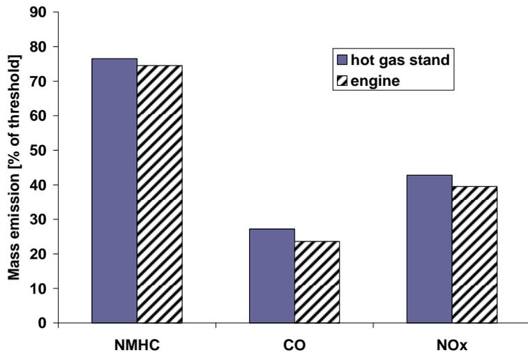
Fig. 9: FTP emission result comparison with different aging methods for ZDAKW catalysts
