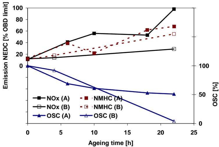
Fig. 16: Comparison of aging methods (A) and (B)
