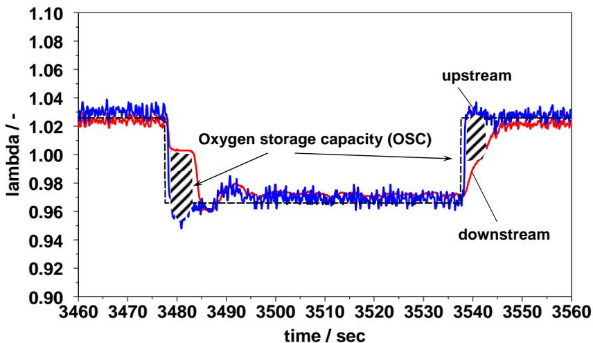
Fig. 14: Oxygen storage capacity measurement on hot gas test stand
