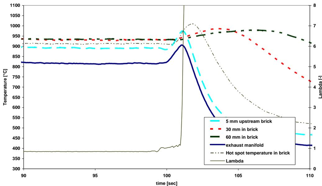
Fig. 7: Shut-off situation measured in a vehicle
