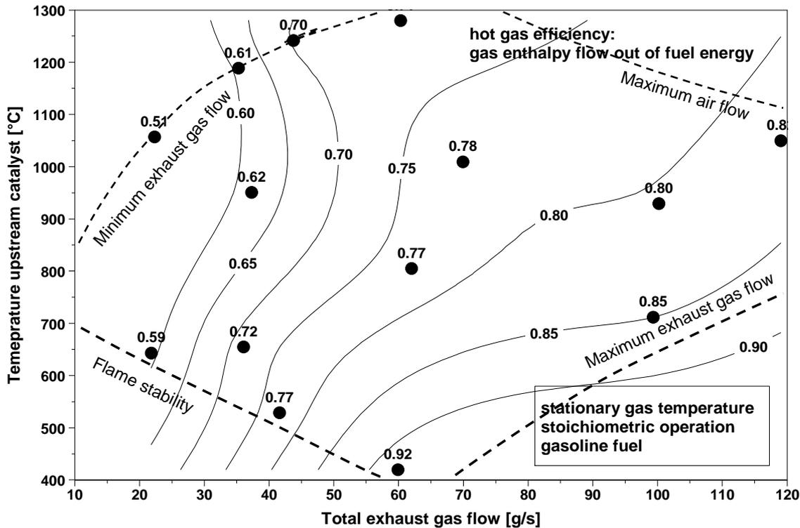
Fig. 4: Hot gas aging bench efficiency map and operation limits
