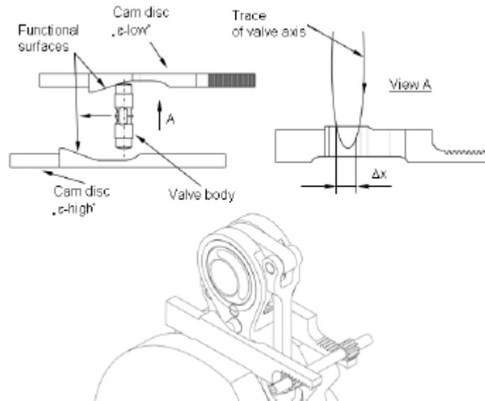
**Figure 10: Actuation with Cam Discs**
