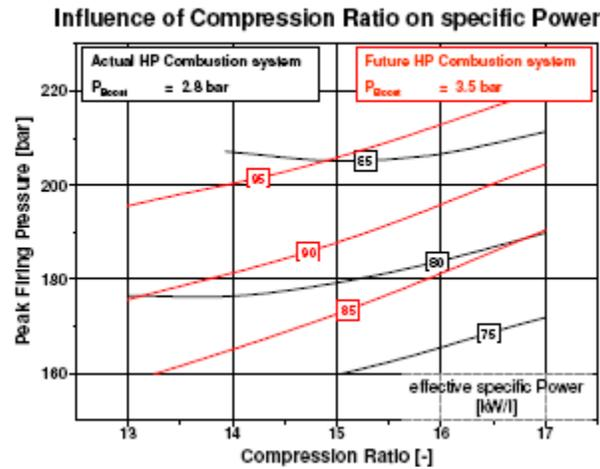
Figure 5: Influence of CR on Peak Firing Pressure and Specific Power Output
