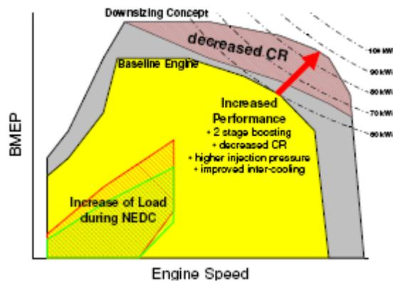
Figure 5: Downsizing Concept with VCR
