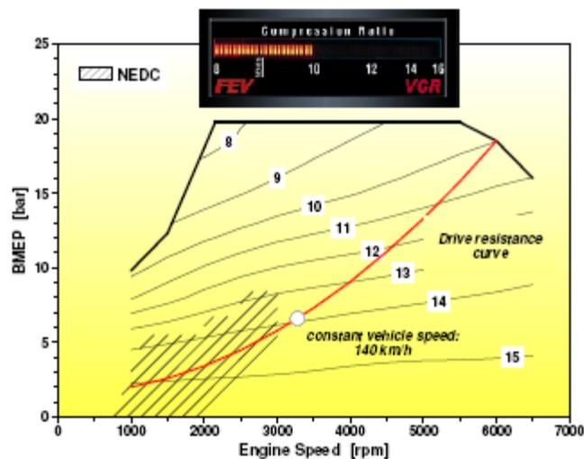
Figure 3: Compression Ratio Operation Map
