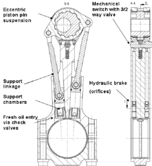
Figure 9: Layout of the VCR Connecting Rod
