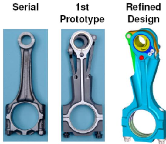
Figure 11: Refined Design for a VCR-conrod for Gasoline Engines
