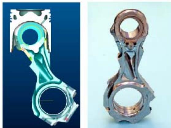
Figure 12: Realized Design of a VCR Connecting Rod for a Truck Application and Prototype
