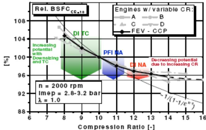
Figure 1: FC Reduction through VCR (Part Load)
