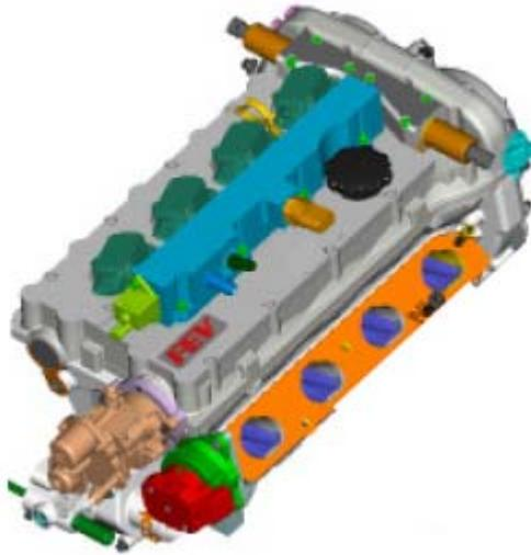
Figure 8: FEV SGT Cylinder Head Design
