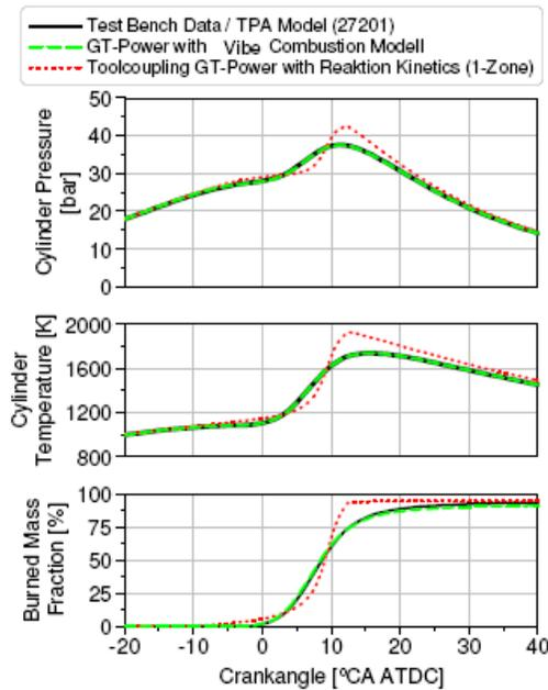
**Figure 7: Comparison of Engine Testing Data with GTPower Results with Vibe and Reaction Kinetics Combustion Rate for CCR Mode at 2000 rpm and 3 bar NMEP**
