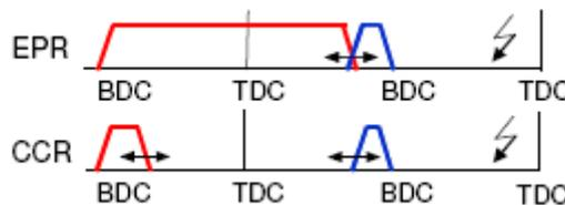
Figure 2: Exhaust Port Recirculation (EPR) and Combustion Chamber Recirculation (CCR)
