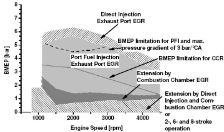
Figure 1: Operating Range of the CAI Strategies Including Direct Injection and Boosting
