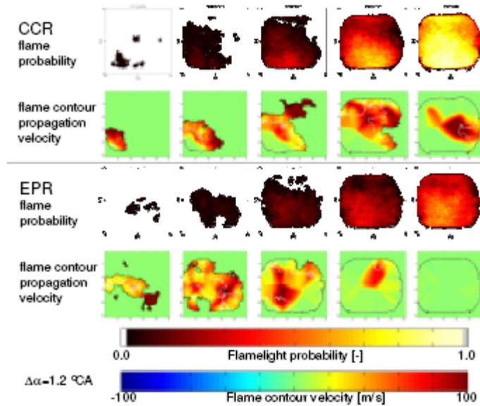
Figure 4: UV- flame Light Evaluation, Providing the Flame Probability and Flame Contour Normal Propagation Velocity
