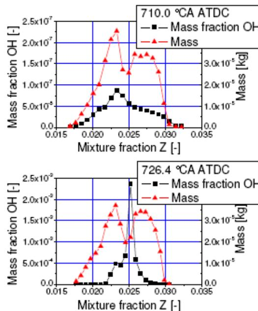
Figure 6: Instantaneous Mixture Fraction and Mass Fraction of OH Radicals at 10 °CA bTDC (ignition) and at 6.4 °CA aTDC (50 % Conversion Point) for CCR Operation
