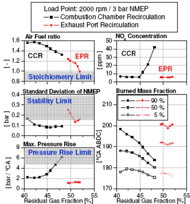
Figure 5: Combustion Characteristics at 2000 rpm and 3 bar NMEP
