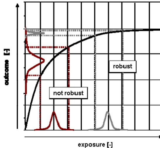
Figure 3 - Influence of exposure variance on robustness according to [9]
