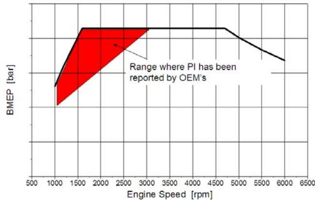
**Figure 1 – Illustration of operation area where pre-ignition events have been reported in turbocharged gasoline engines.**
