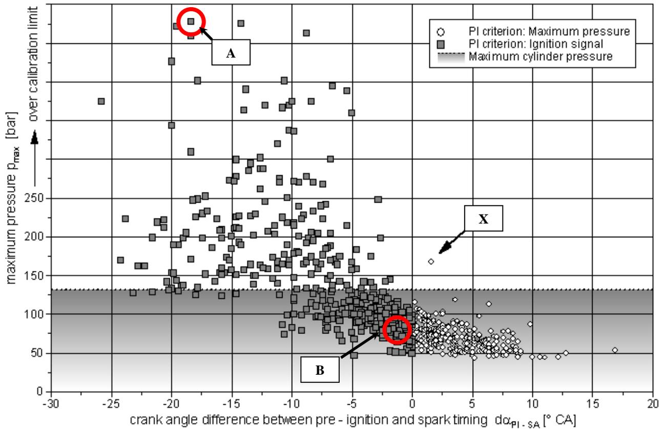
**Figure 13 - Pre-ignition maximum pressures with different detection criteria**
