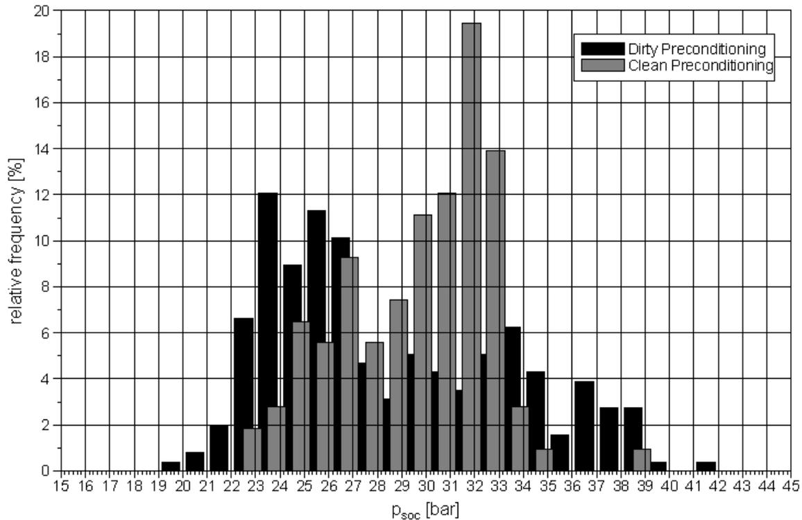
**Figure 11 - Pressure at start of combustion for dirty versus clean pre-conditioning**
