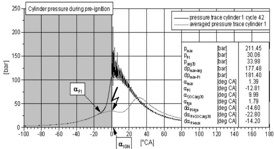
**Figure 12 - Pre-ignition detection criterion**
