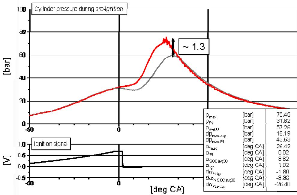
Figure 16 - Example for a modest pre-ignition event (B), test run settings: # 6 after clean pre-conditioning
