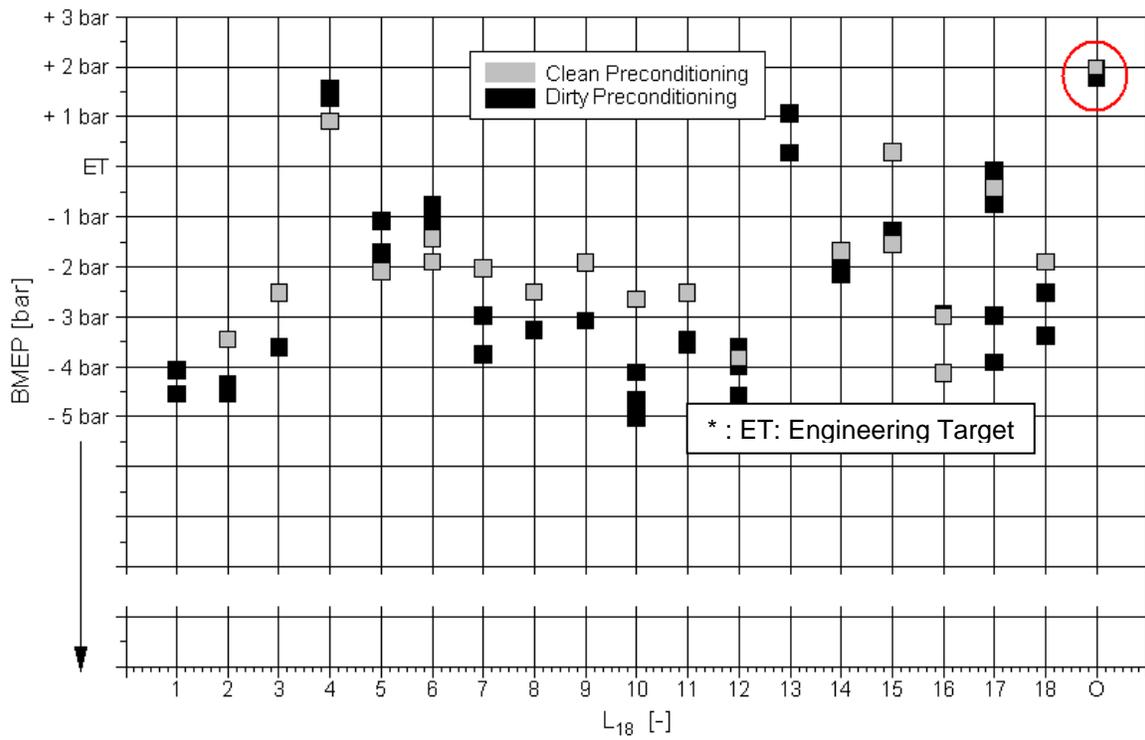
**Figure 10 - BMEP level at first pre-ignition occurrence for the different L18 test run settings**
