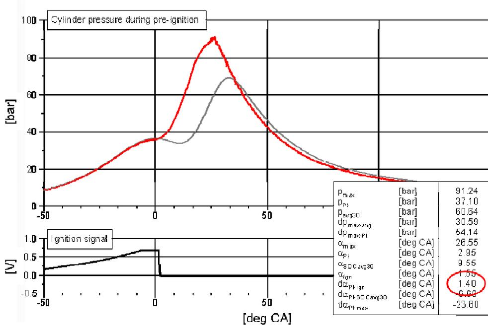
Figure 17 - Example for a pre-ignition event occurring shortly after spark ignition during burning delay, test run settings: Validation point after clean pre-conditioning
