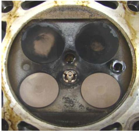
**Figure 9 - Combustion chamber roof after “clean” conditioning (on top) vs. “clean” followed by “dirty” conditioning (underneath)**
