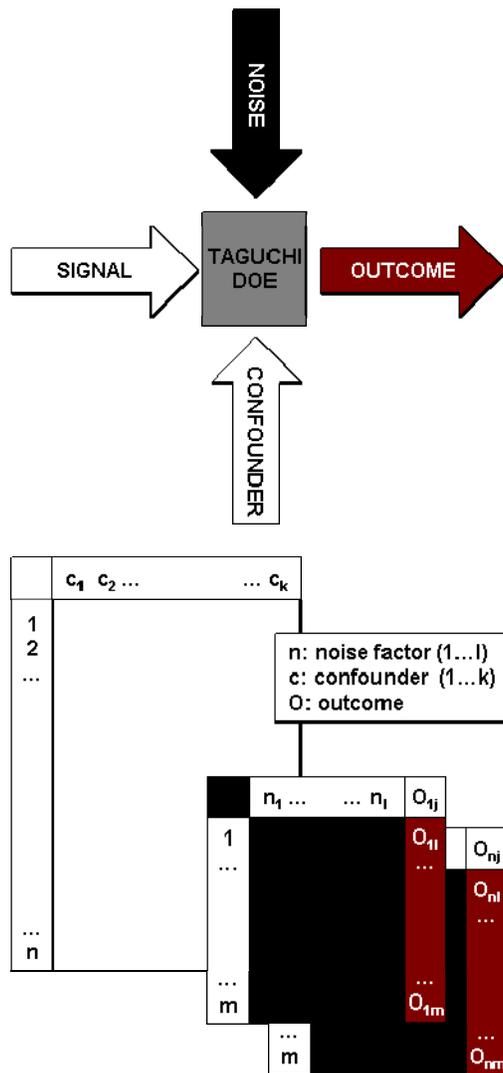
Figure 5 - General setup of an experimental design according to Taguchi
