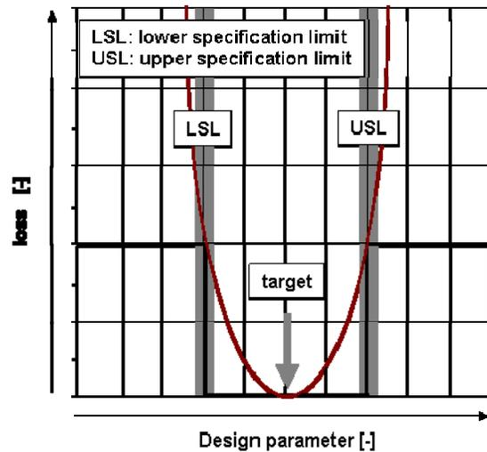
Figure 4 - Quality loss according to Taguchi
