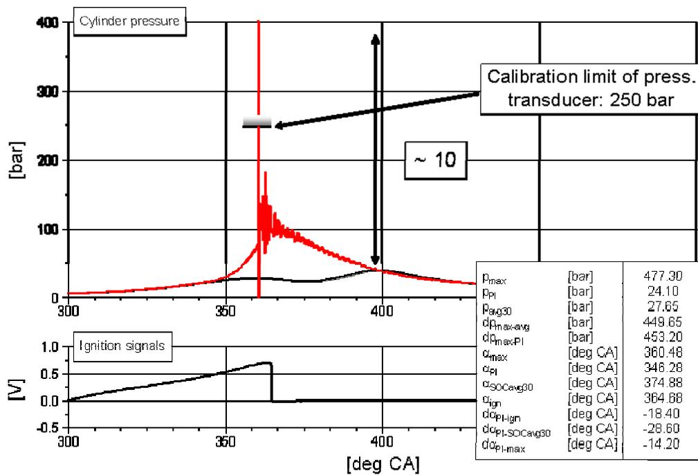
Figure 15 - Example for a severe pre-ignition event (A), test run settings: # 9 after dirty pre-conditioning
