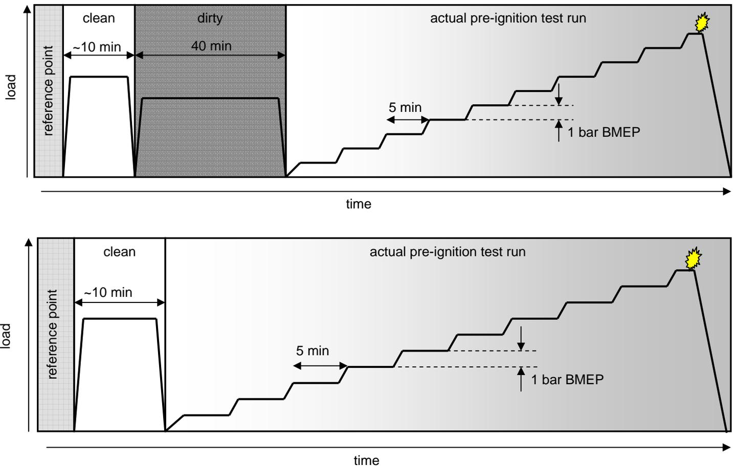
Figure 6 - Sequence of one L18 test run with reference point check and pre-ignition test in comparison (upper) with “clean” and “dirty” conditioning vs. (lower) only “clean” conditioning
