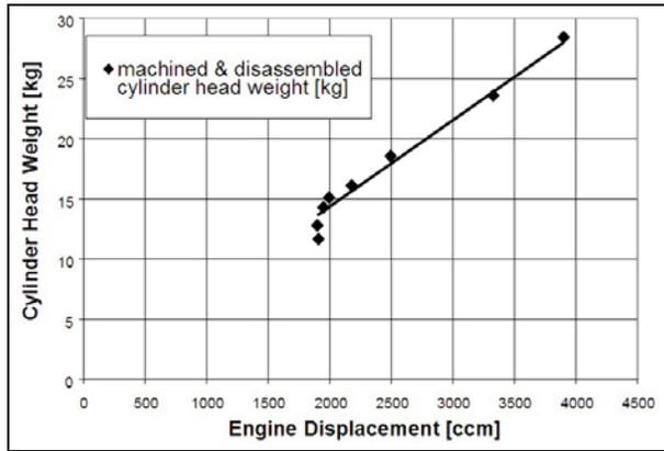
Figure 2: Comparison of Cylinder Head Weight (Aluminum)
