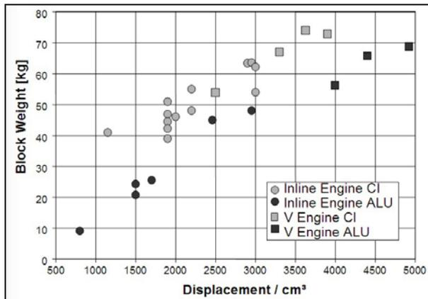
Figure 3: Comparison of Block Weight (HSDI Engines)
