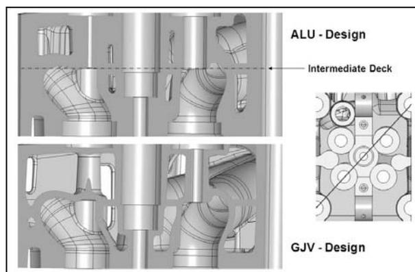
Figure 7: Cast Iron Design versus Aluminum Design
