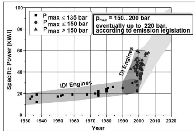
Figure 1: Specific Power and Peak Firing Pressure
