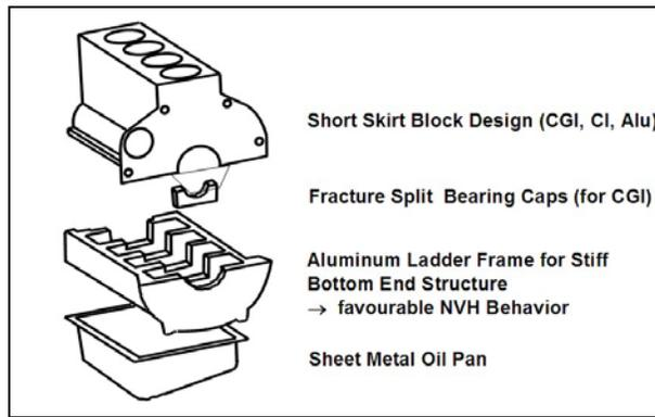
**Figure 9: Lightweight Bottom End Concept**
