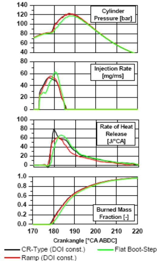
Figure 8: Variation of Injection Shape at 228rpm, 9.4 bar IMEP, SOI: 7°CA bTDC, EGR-Rate: 27%
