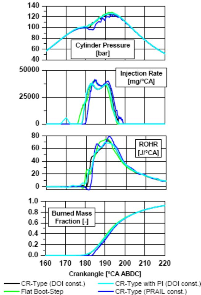
Figure 6: Variation of Injection Shapes at 2400 rpm, 14.7 bar IMEP, Center of Combustion: 14°CA aTDC, EGR-Rate: 22%
