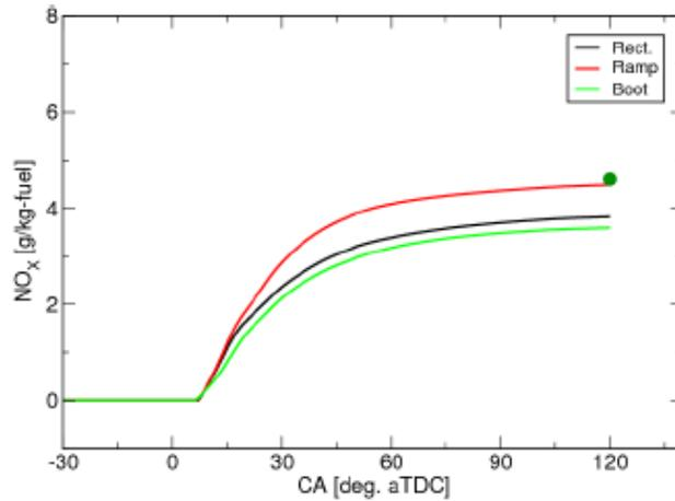
Figure 17: Comparison of NO<sub>x</sub> emission
