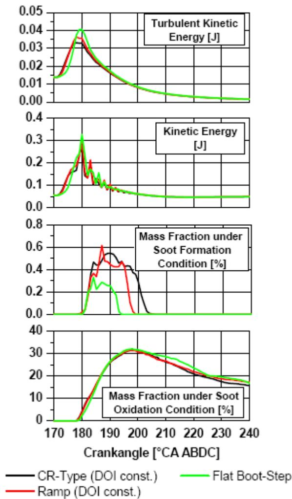
Figure 12: Summary of KIVA Results at 2280 rpm, 9.4 bar IMEP
