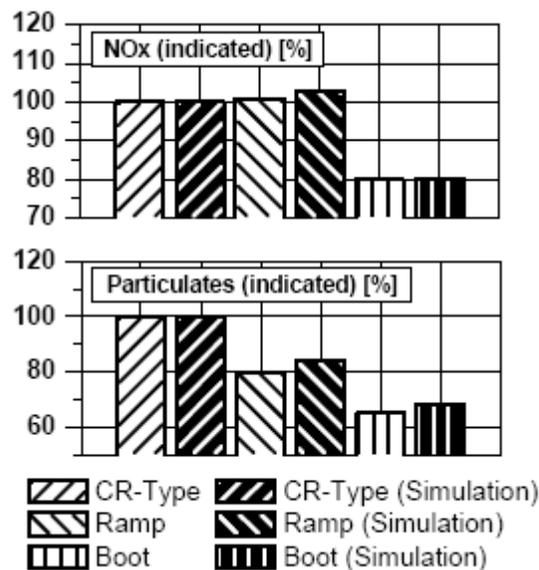
Figure 9: NO<sub>x</sub>- and Soot Emission at 2280 rpm, 9.4 bar IMEP, SOI: 7°CA bTDC, EGR: 27%
