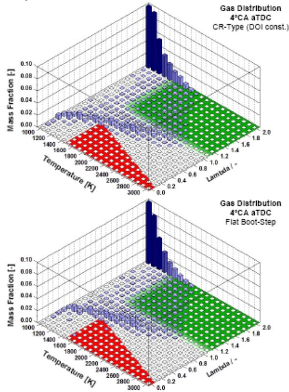
Figure 10: Gas Fraction 4°C aTDC at 2280 rpm, 9.4 bar IMEP, SOI: 7°C aTDC, EGR: 27%
