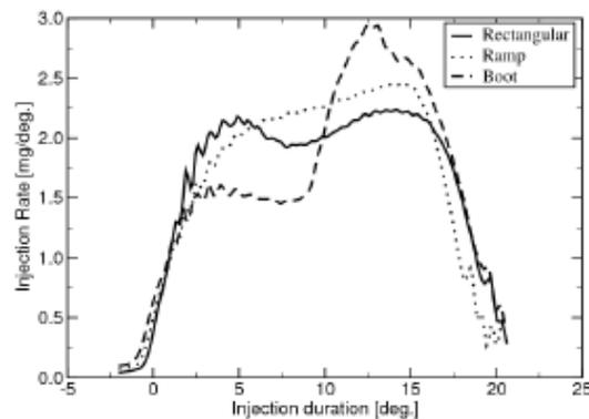
Figure 13: Injection Rate Shapes
