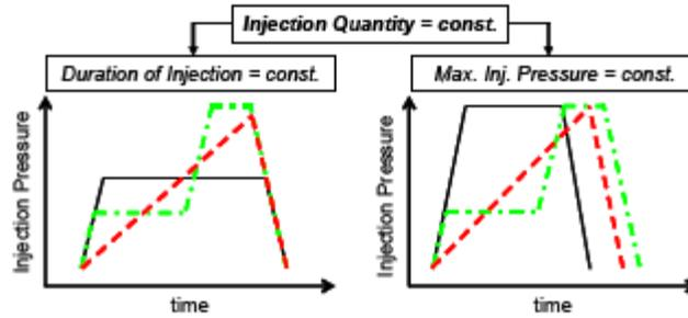
Figure 4: Measures for constant injection quantity
