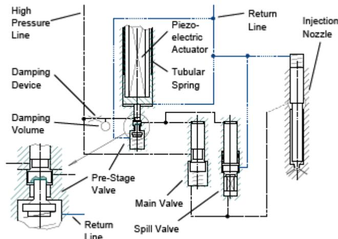
Figure 3: Scheme of CoraRS Setup
