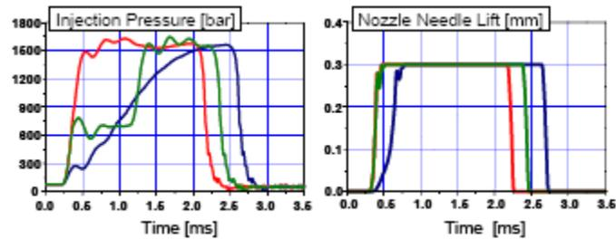
Figure 2: Rate Shapes on the Injector Test Bench
