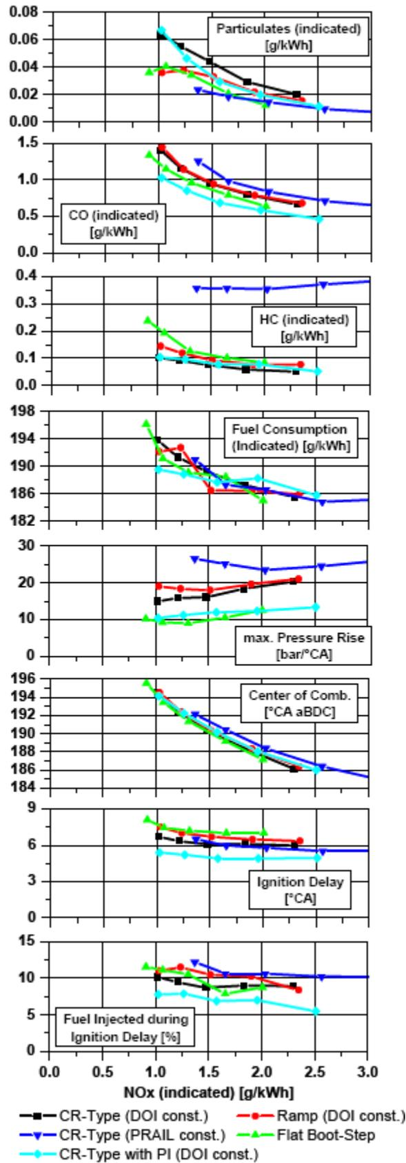
Figure 7: Variation of Injection Timing (7 to -1°CA bTDC) at 2280 rpm, 9.4 bar IMEP, EGR-Rate: 27%
