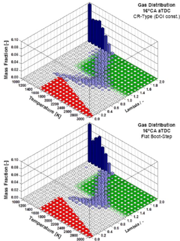
Figure 11: Gas Fraction 14°C aTDC at 2280 rpm, 9.4 bar IMEP, SOI: 7°C aTDC, EGR: 27%
