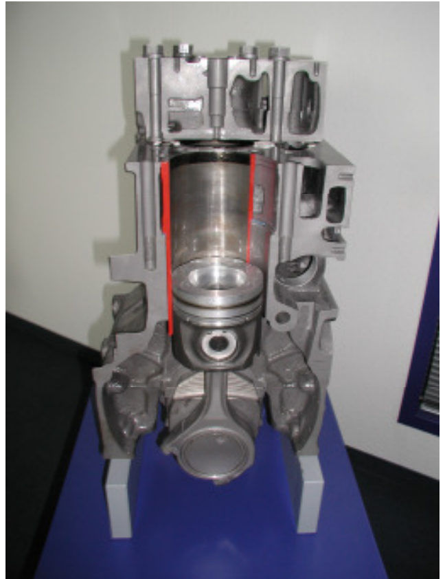
Medium Duty Engine with open-deck crankcase
