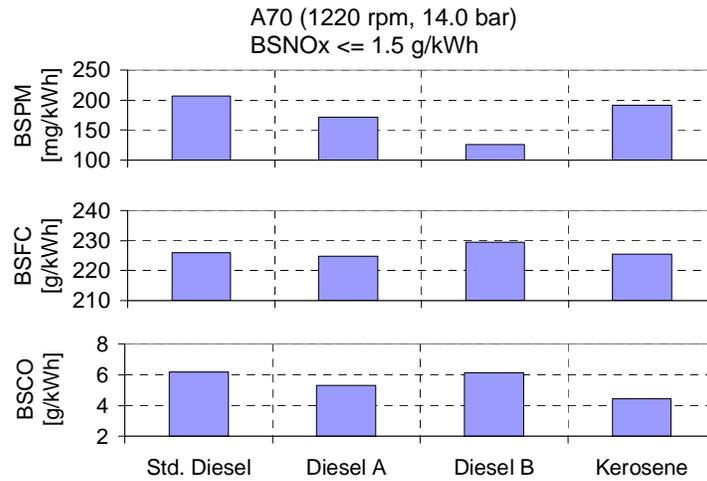
Figure 15: DOE optimized comparison of the A70 load point under part homogeneous operation
