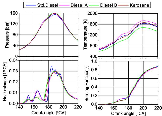
Figure 16: Heat release of the A70 load point under part homogeneous operation
