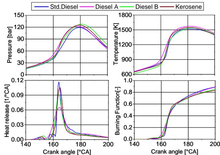
Figure 14: Heat release of the A25 load point under part homogeneous operation
