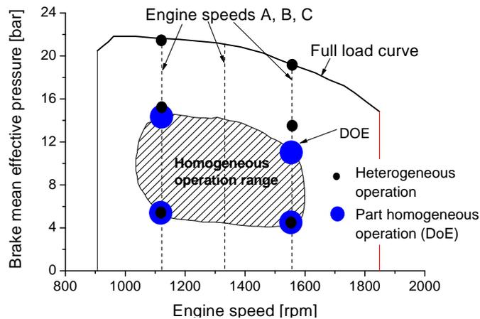
Figure 9: Engine operating points for fuel testing
