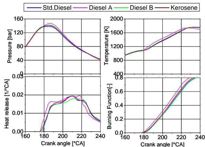
Figure 12: Heat release analysis of the full load point (C100) under heterogeneous operation
