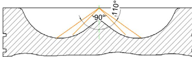
Figure 6: Piston bowl geometry
