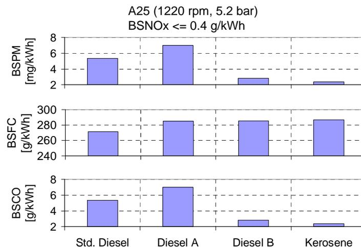
Figure 13: DOE optimized comparison of the A25 load point under part homogeneous operation
