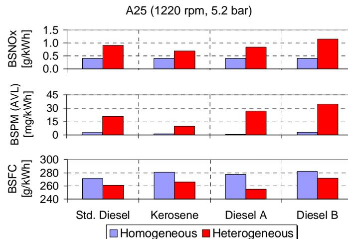
Figure 17: Emission comparison between heterogeneous and part homogeneous combustion
