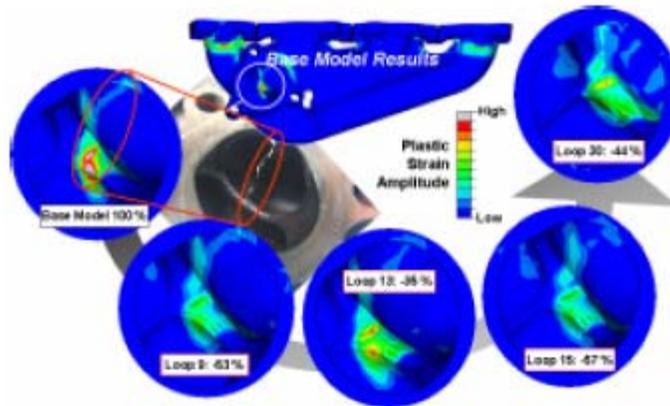
Figure 7: Plastic Strain Optimization (Global Model)
