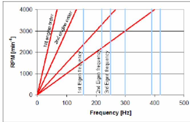
Figure 5: Engine Speed Over Eigen Frequency
