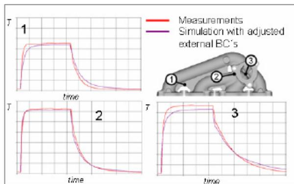
Figure 4: Transient Thermal Analysis Results
