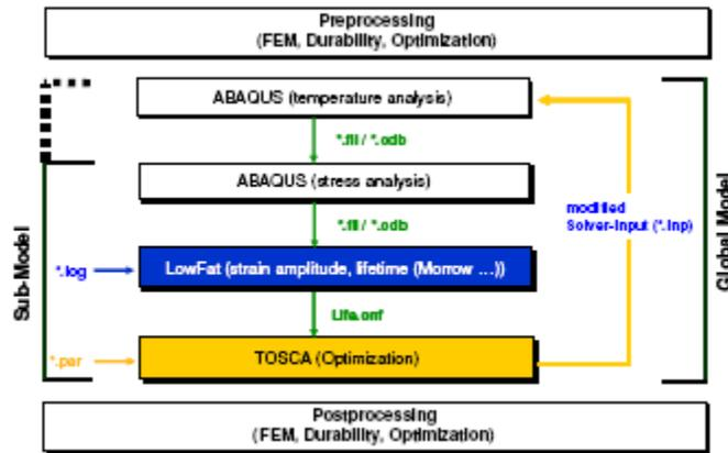
Figure 6: Closed Loop Optimization
