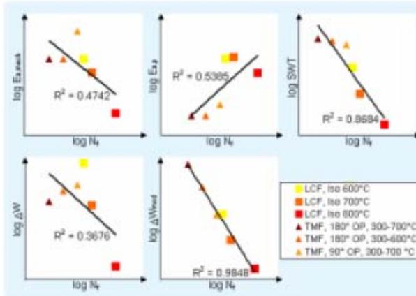
Figure 3: Correlation of Damage Indicators to High Temp. Isothermal and Thermomechanical Results of GJS-SiMo
