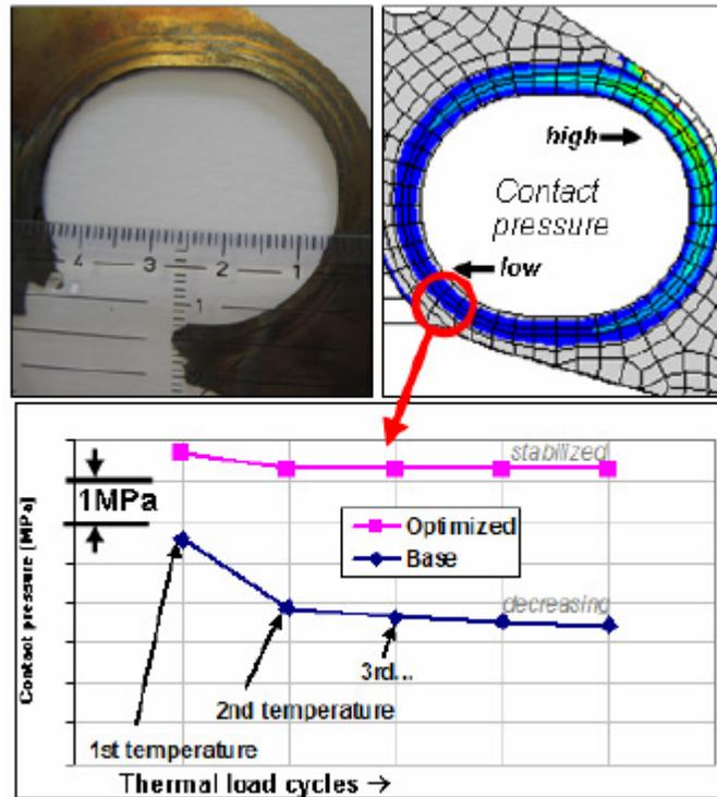
Figure 8: Gasket Leakage
