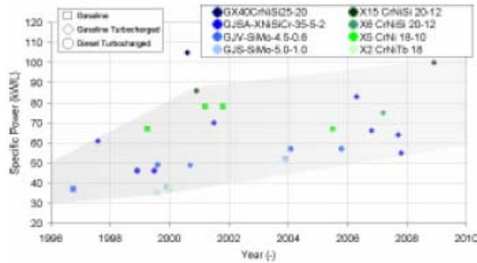
Figure 1: Exhaust Manifold Material Benchmark
