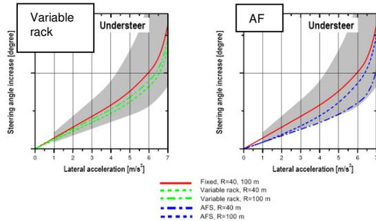
Figure 5: Influence of Variable Rack and AFS on Understeer Gradient
