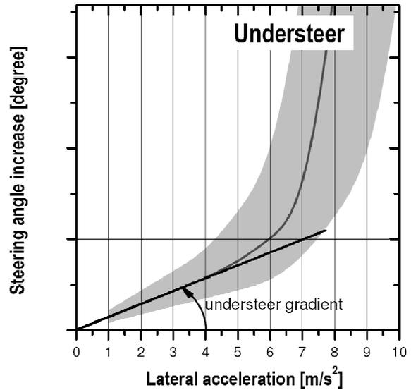
Figure 4: Typical under steer behaviour
