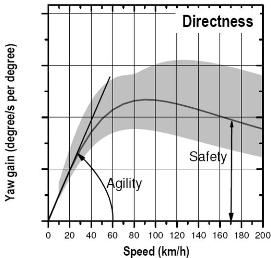
Figure 1: Traditional Relation Between Agility and High Speed Safety
