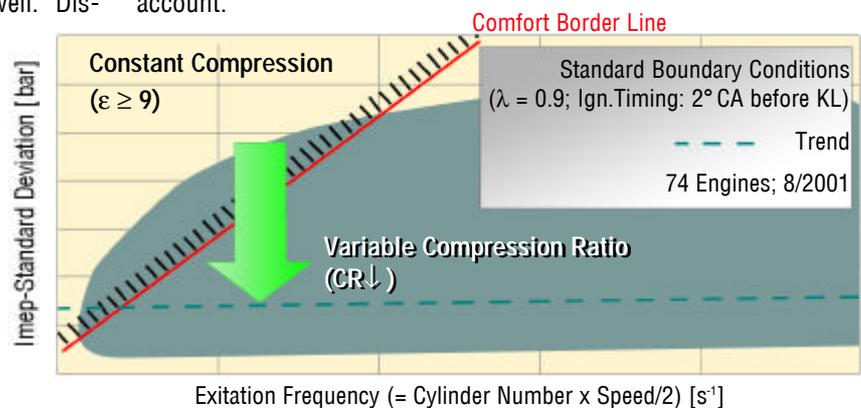
Here, the use of variable compression ratio (VCR) leads to the possibility of combining optimized torque characteristics with the best possible part load fuel consumption.
