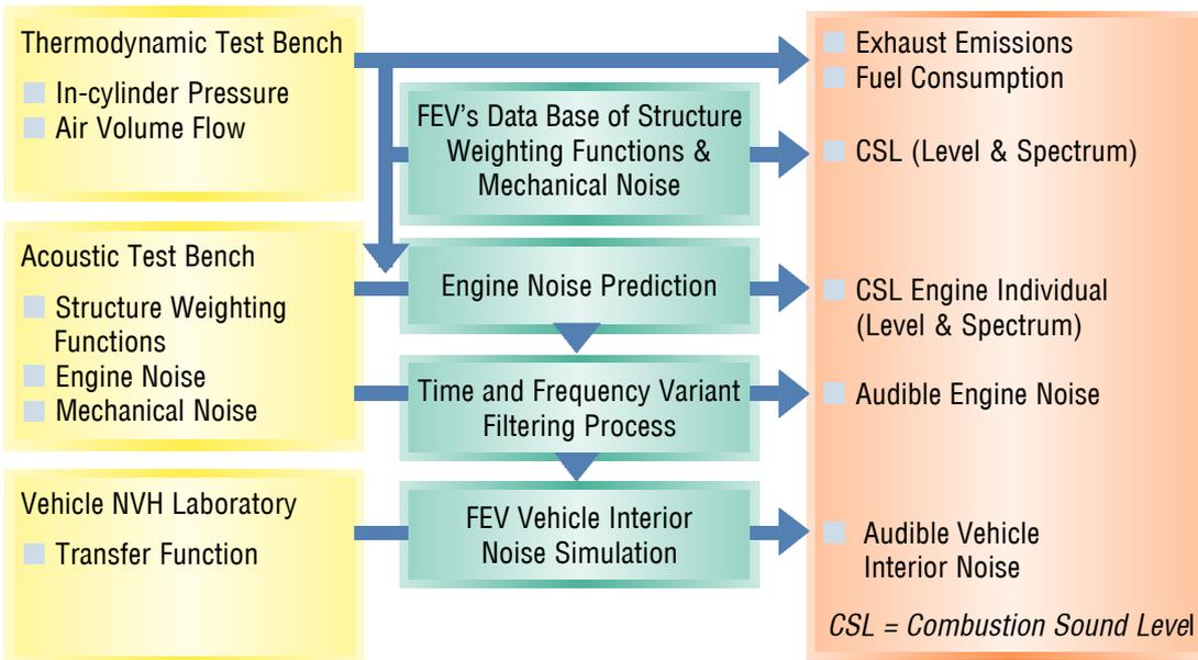
FEV's in-cylinder pressure based noise prediction tools
