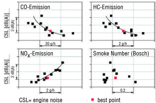
of the “best point” achieved for idle at cold start condition (<< 20°C) for a direct-injected Diesel engine.
