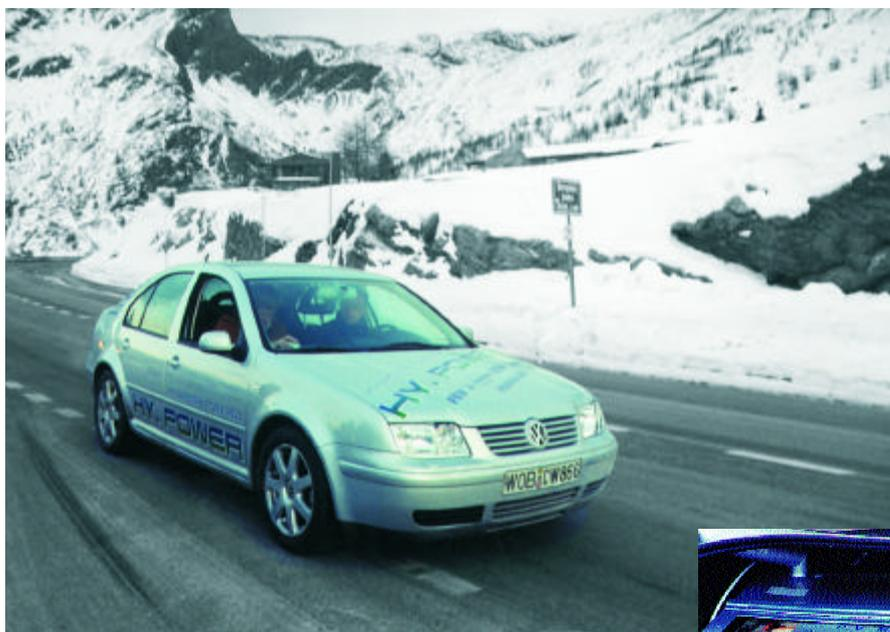
The Paul-Scherrer Institute and FEV Motorentchnik GmbH in close cooperation with Volkswagen AG have developed a hybrid electric demonstrator vehicle with fuel cells and supercapacitors. The vehicle delivers the targeted brake energy recovery and provides sufficient performance.
