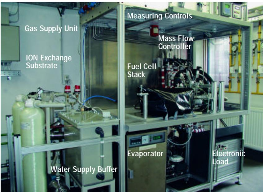
Control and data acquisition are achieved through the implementation of the ADAPT process control system with integrated SPS. The control unit may be connected with a Matlab/Simulink based system simulation tool to perform in-the-loop testing of the stack under real-life, reproducible and transient operating conditions.
