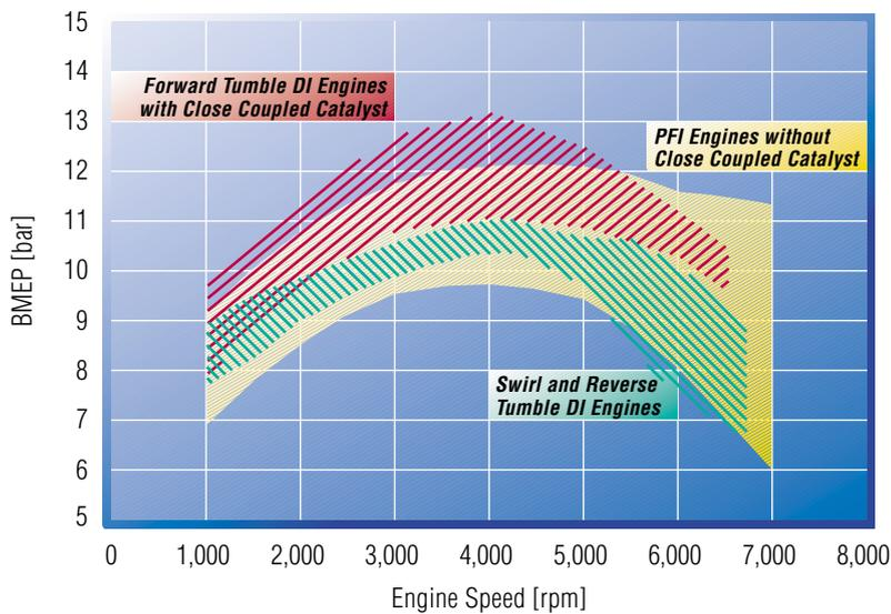
DI combustion processes with low HC raw emissions is high, and therefore has recently been established as an essential development target. This shows that combustion systems like FEV's air-guided concept, which include minimal wall wetting of the injected fuel, have an additional advantage.
