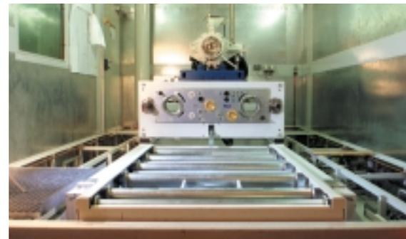
The modules are suitable for engines up to 500 kW including their auxiliary components.
