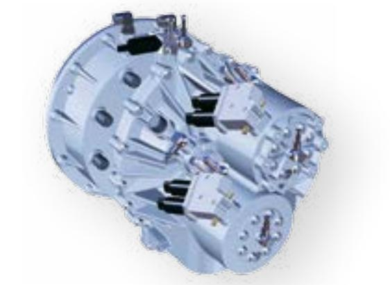
Fig. 9: FEV 7-speed hybrid powershift transmission
