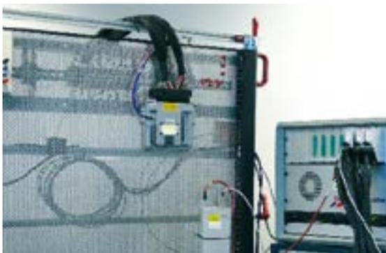
*Fig. 4: HIL Testbench for TCU testing and calibration*
