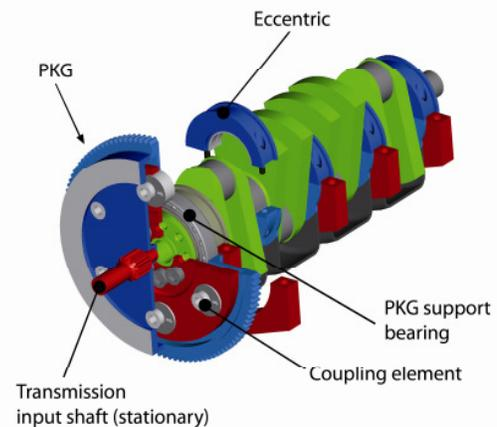
Fig. 2: Design of the VCR system
