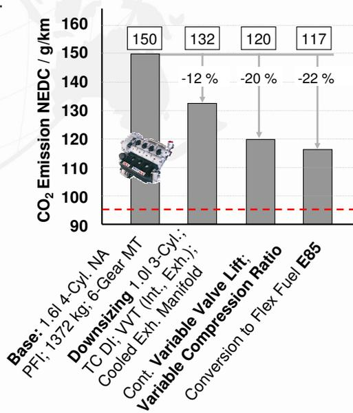
Fig. 1: Example scenario of CO<sub>2</sub> saving potential of VCR in combination with downsizing
