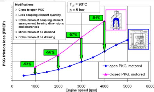
Fig. 3: Progress in PKG friction reduction
