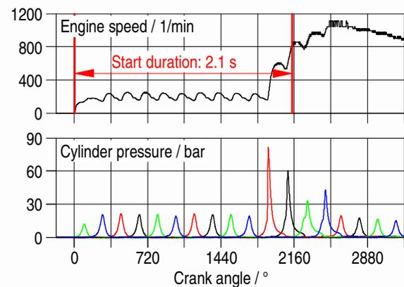
Fig. 2: E100 cold start calibration of FEV SGT engine for - 10 °C ambient temperature
