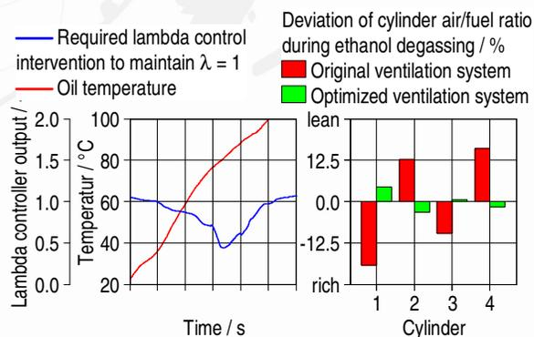
Fig. 5: Degassing of ethanol from lube oil during engine warm-up after repeated cold starts and blow-by system optimization
