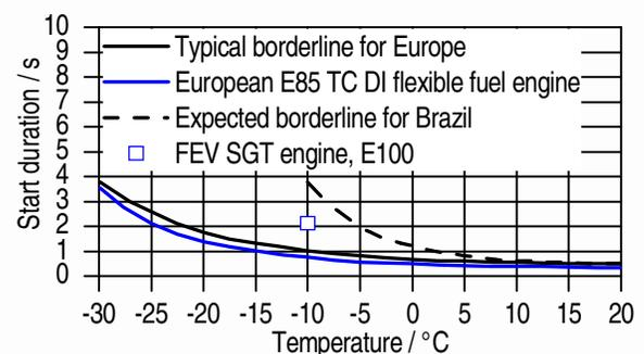
Fig. 3: Starting times for cold start
