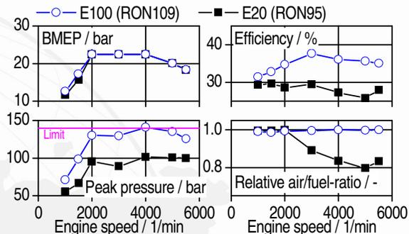
Fig. 4: Full load of FEV SGT engine with E100 and E20
