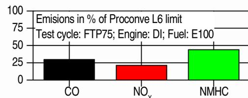
Fig. 6: Emissions of the SGT DI engine in the FTP75 test cycle using E100
