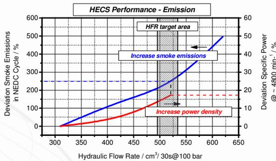
Fig.1: Assessment of power density and PM emissions vs. hydraulic flow rate ( $p_{max} = 200$  bar)
