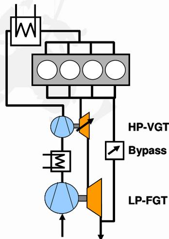
Fig.2: Two stage serial turbo-charging architecture for achieving highest power density
