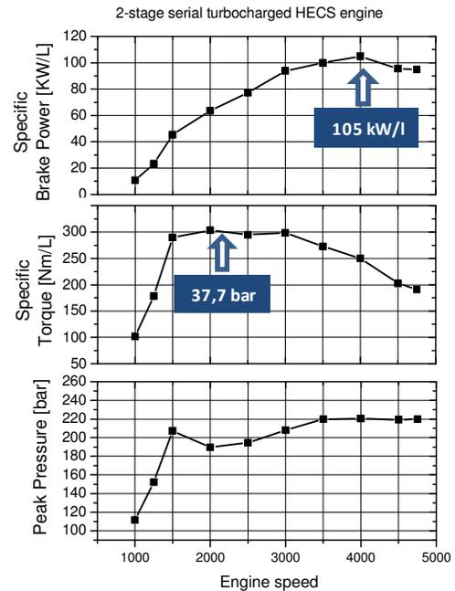
Fig.3: Balance between peak firing pressure and specific power output (Full Load Point @ 4000 rpm)
