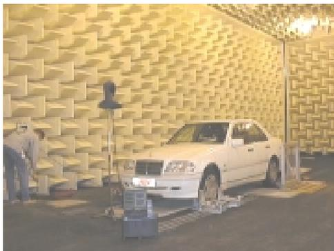
FEV conducts extensive **NVH benchmarking** on vehicles in order to continually assess the state of the art. NVH relevant design features are analyzed and various metrics stored in a proprietary database. Such a database helps identify areas of weakness in a given vehicle and provides guidance for **NVH target setting**.
