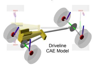
spect to torsional and bending resonances by using CAE tools. As part of driveline development attention is focused on transient events as well as on harmonic behavior.
