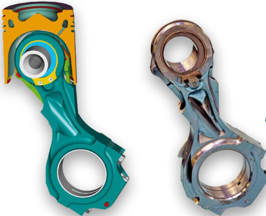
*Fig. 5: Realised design of a VCR-conrod for a heavy duty diesel application and prototype*
