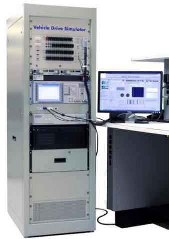
TST with complete simulation and model based operating software
