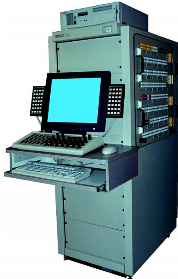
The system has several bays for customized load trays meeting the I/O requirements of various ECUs. These trays are easily removed and mate to a system interconnect board. The interconnect board provides a convenient routing mechanism for the large number of interconnection points for various higher pin count ECUs.
