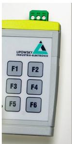
For this application the Baby-LIN-RC (on the left) with its integrated key pad will be a good and economic choice. As it can be operated stand alone, it will only be connected to the LIN bus, no PC connection will be necessary!
