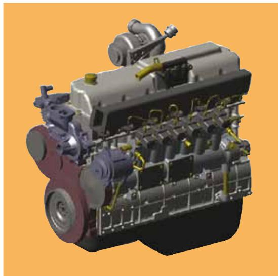
A major target was to carry over as many features as possible from the F6108, in order to minimize the investment required for production facilities. The existing machining line for the crankcase defined the bore spacing for the new engine.
