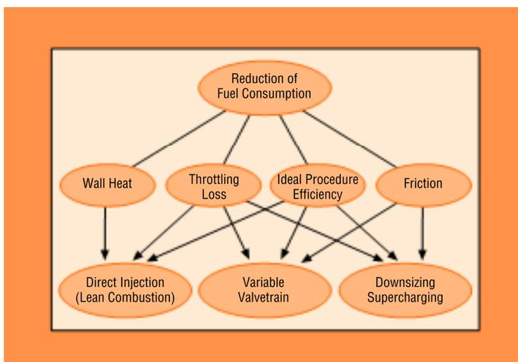
Gasoline engine concepts that can be utilized for the reduction of fuel consumption are illustrated in Figure 1. Direct injection with lean combustion causes minimal wall heat losses. Partial and fully variable valvetrains reduce pumping losses through dethrottling.
