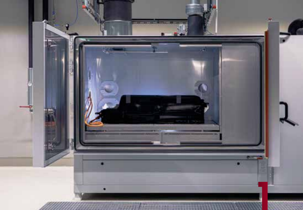
1 Insights from eDLP test stands. 1. Climatic chamber with energy system / 2. IPX-waterjet / 3. 350-kN shaker with temperature chamber and energy system.
