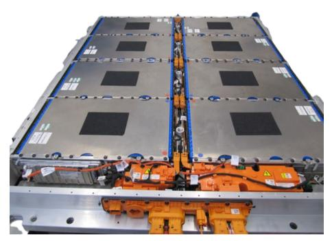
**Caption:** Outstanding performance and fulfillment of highest safety standards for Indian Electric Origin vehicles: Mahindra and FEV have jointly developed an innovative battery system available with a total capacity of 59 or 79 kWh. Source: FEV/Mahindra
