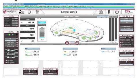
Dashboard example of MORPHEE – the unique software solution for control and automation of test benches is now also adapted to the special needs of emobility solutions.
