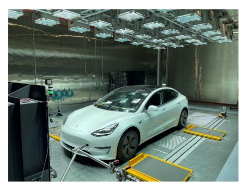
The new solar simulation system plays an important role for globally applicable regulatory tests of both electric vehicles and vehicles with an internal combustion engine.
