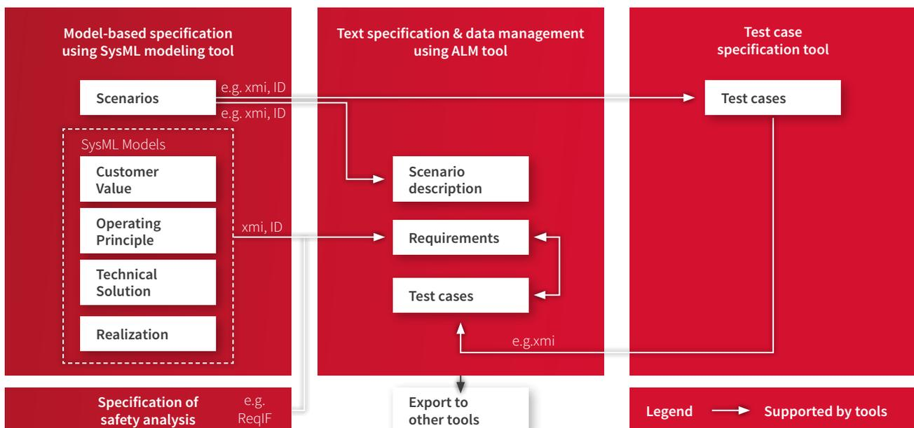
© Possible generic tool chain for supporting the scenario and model-based systems engineering process all the way up to testing
