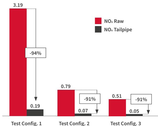
⑤ Simulated SCR efficiencies and resulting tailpipe emissions for an SCR only aftertreatment system
