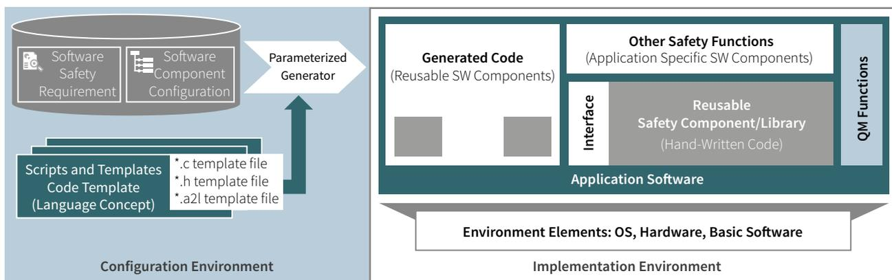
② Parameterized code generation for reusable software components: The development of these is performed by using a tailored tool chain which supports configuration selection, configuration validation, as well as parameterized code generation.
