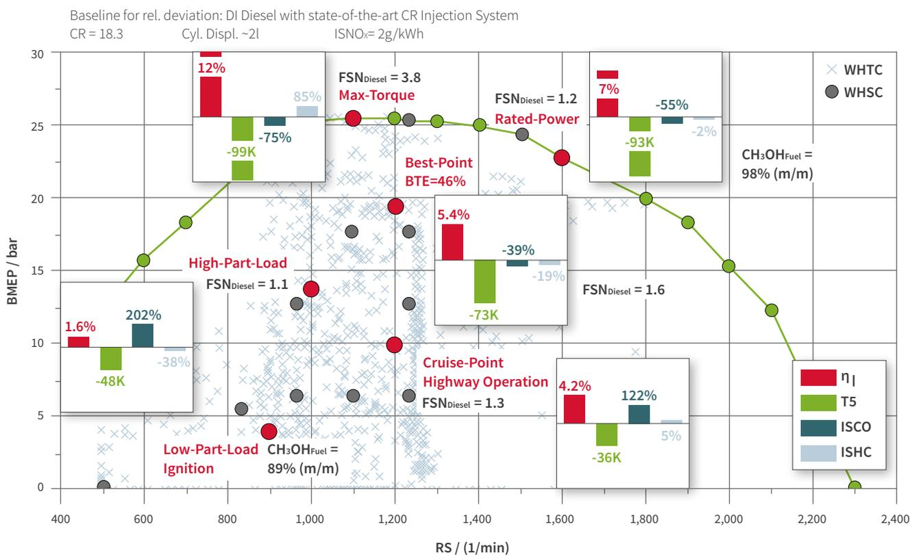
The comparison of diesel and methanol DDI CI under iso-ISNO<sub>x</sub> conditions rounds off the differences between both combustion modes. A comparison at ISNO<sub>x</sub> = 2 g/kWh is chosen to consider future emission standards. This comparison is performed for several operating points in Figure 2.
