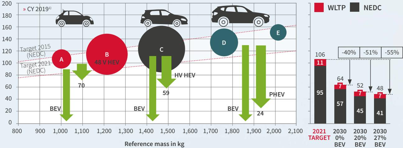
④ Segment specific and fleet averaged EU passenger car NEDC CO<sub>2</sub> emission targets (WLTP considered with a mark-up) for 2021 and outlook to 2030 considering only gasoline (P)HEV and up to 27 percent BEVs
