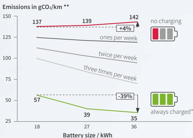
⑤ Impact of battery sizing and battery charging behavior on real-world CO<sub>2</sub>/fuel consumption
