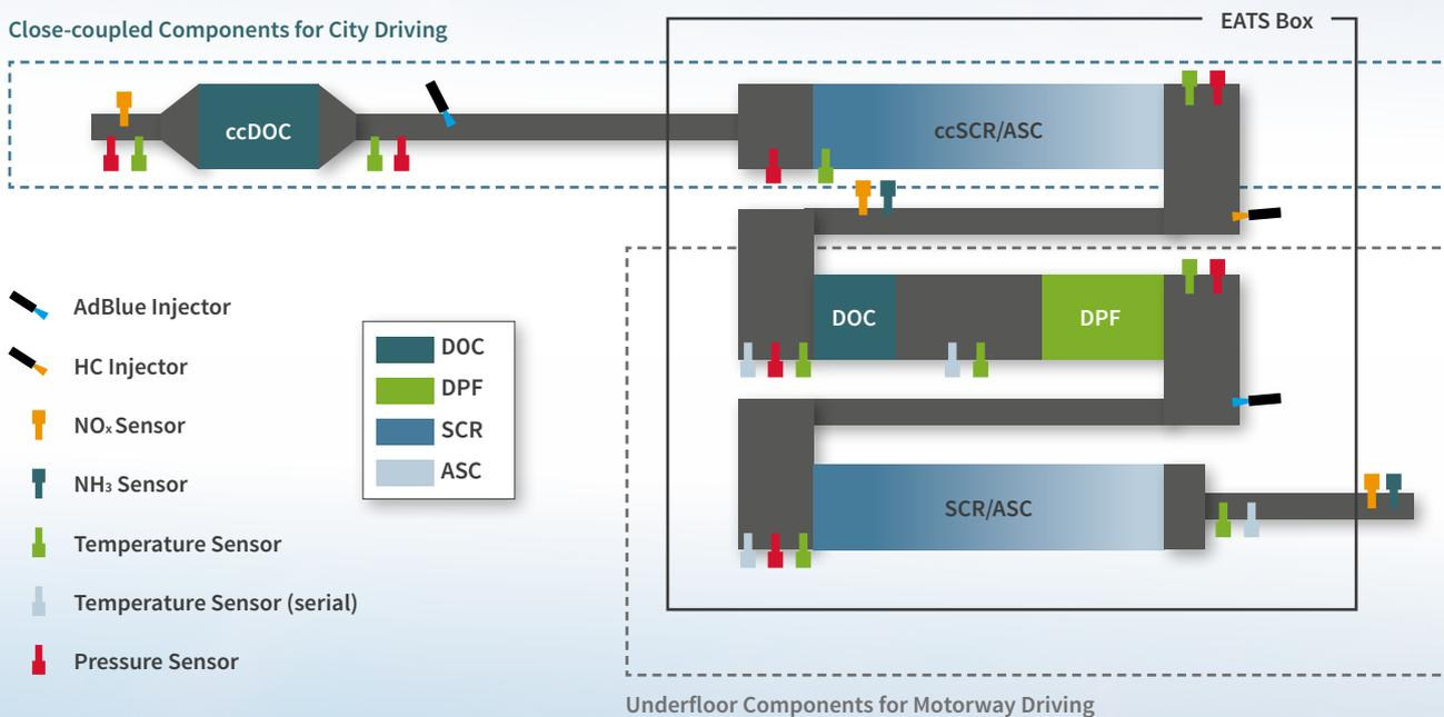
③ Schematic layout of EATS including sensor setup
