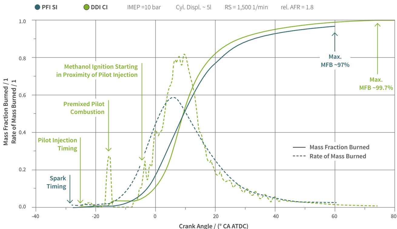
④ Mass fraction burned for methanol DDI CI and PFI SI
