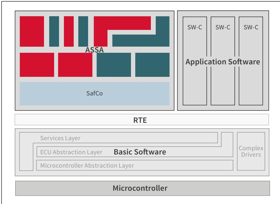
① An ASSA-based safety-critical software integrated in an AUTOSAR control unit software. The Safety Coordinator encapsulates all safety software components which consist of reusable and application-specific components.
