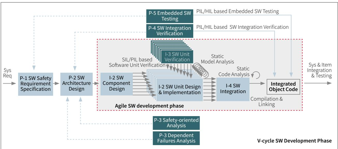
③ Overview of ASSDP. Waterfall and agile phases are interlaced in order to introduce more iteration- and increment-based phases in the safety-critical software development. For each phase the different process steps are presented with their logical sequence.
