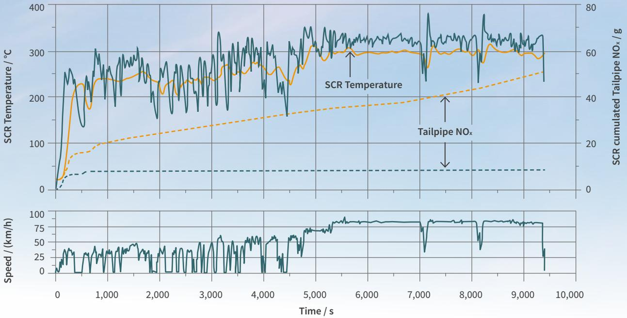
© SCR temperature and NO<sub>x</sub> emissions of the close-coupled SCR vs the EU VI baseline SCR in a simulated ISC trip
