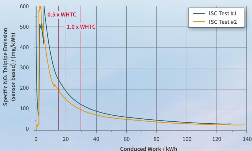
© Cumulative specific tailpipe NO<sub>x</sub> emissions for an ISC trip
