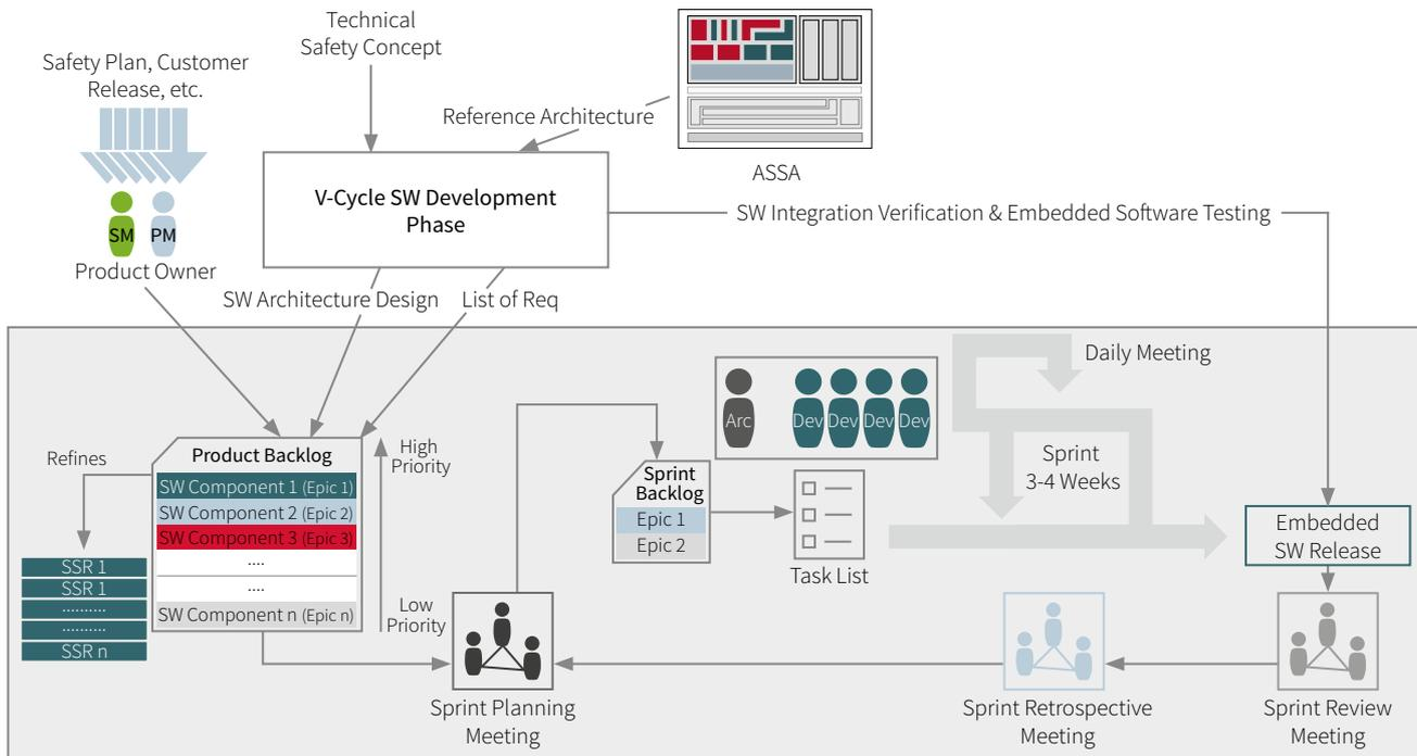
④ *The agile phase of ASSDP. Short and repeated iterations are the core property of this phase which usually last about three to four weeks. Well-known organizational elements from agile software development are used here.*
