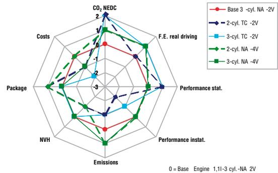
Fig. 4: Overall Evaluation of 2- and 3-Cylinder Concepts
