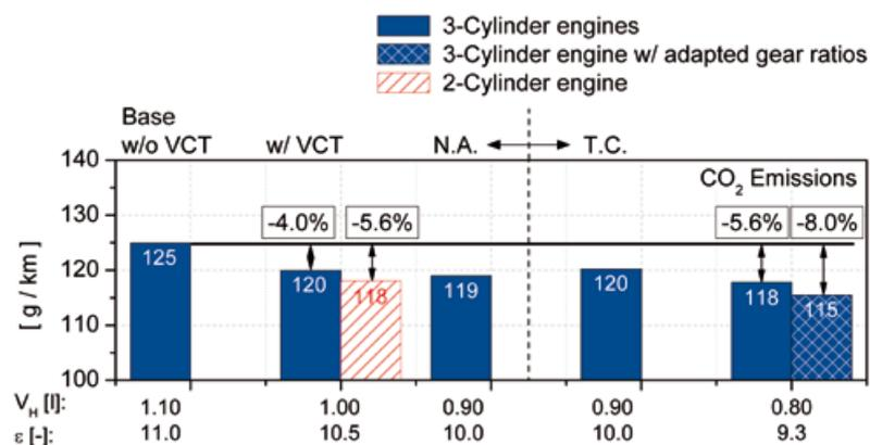
Fig. 3:  $\text{CO}_2$  Emission Reduction in NEDC – Charged and N.A. Variants
