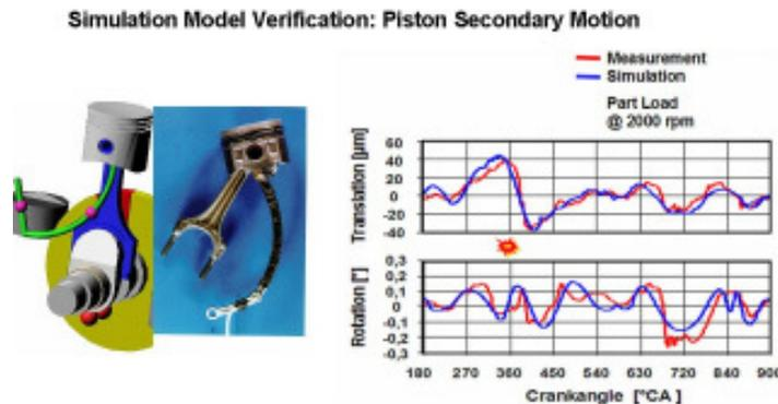
Figure 8: Comparison of Measured and Calculated Piston Secondary Motion
