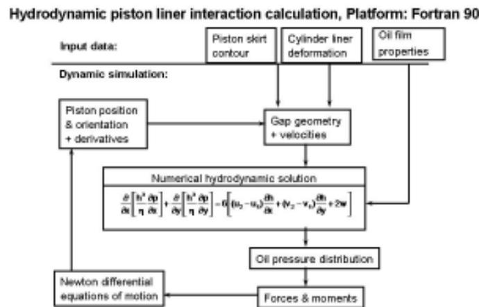
Figure 5: Single Purpose Piston Secondary Motion Simulation Program
