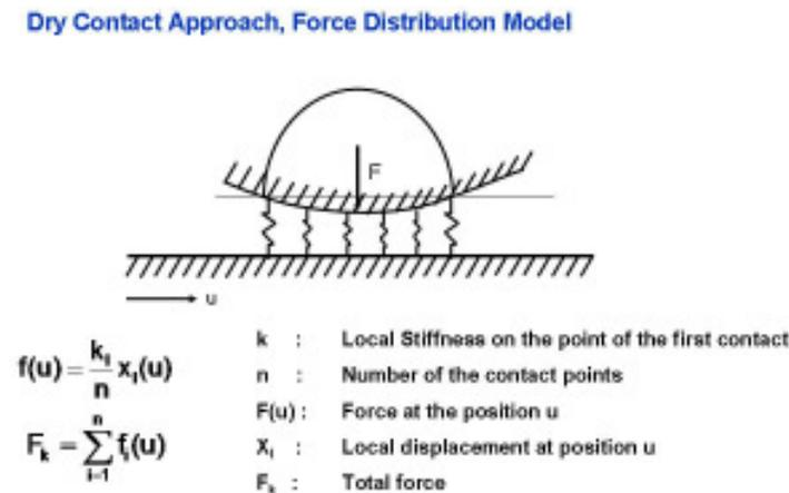
Figure 4: Force Distribution of Dry Contact Model
