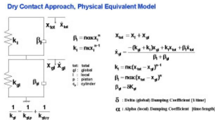
Figure 3: Global and Local Stiffness and Damping of Dry Contact Model
