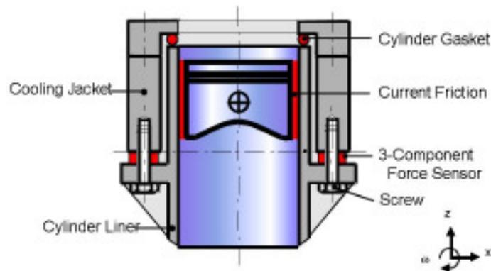
Figure 2: Measurement Setup for Piston group Friction under Fired Conditions [7]
