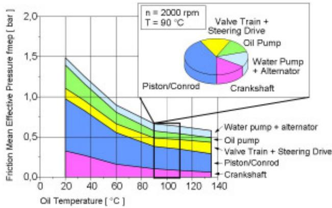
Figure 1: Friction Source Quantification for a 2.0L Gasoline Engine [7]
