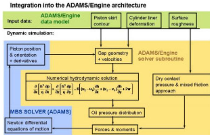
Figure 7: Calculation Procedure for Hydrodynamic Piston Liner Contact Embedded in ADAMS/Engine
