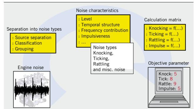
❶ Procedure for computing objective parameters
