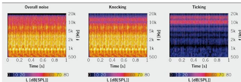
④ Separating the noise of a diesel engine into noise types
