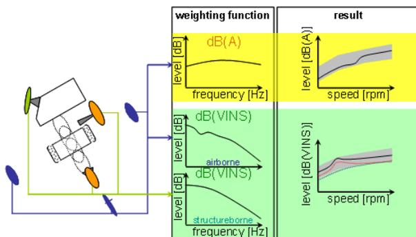
Figure 2: dB(VINS) process for powertrains
