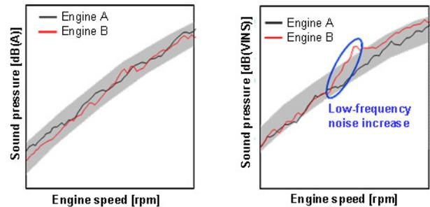
Figure 3: Radiated engine noise level and estimation of interior noise of two different I4 engines with dB(VINS) [3]
