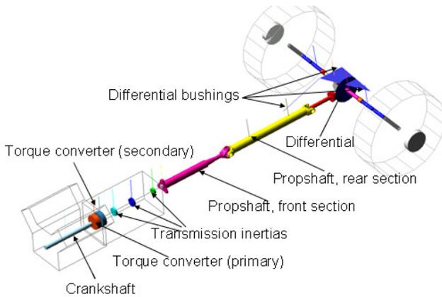
Figure 5: Multi body simulation model for driveline torsional vibration (boom)
