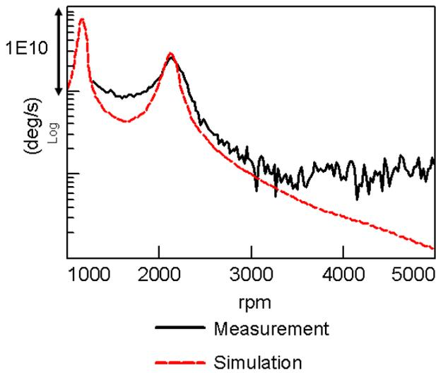
Figure 8: 4<sup>th</sup> engine order correlation of propshaft torsional vibration (close to axle input) between measurement and simulation for WOT run-up in 2<sup>nd</sup> gear
