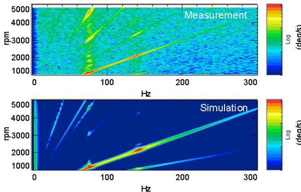
Figure 9: Spectral map information of measurement and simulation for propshaft torsional vibration (close to axle input) for WOT run-up in 2<sup>nd</sup> gear
