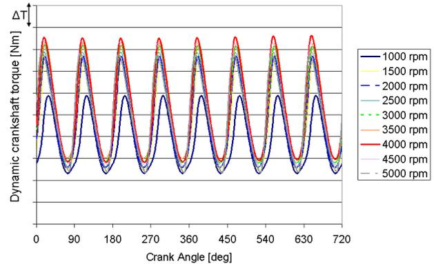
Figure 7: Dynamic crankshaft torque for a V8 naturally aspirated gasoline engine at WOT for different engine speeds
