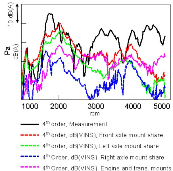
Figure 4: Comparison between measured interior noise levels and dB(VINS) prediction of the structure borne noise paths
