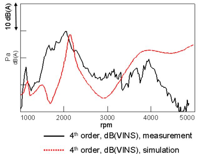
Figure 12: Comparison of interior noise share for rear axle boom between measured and simulated rear axle vibration for 3rd gear
