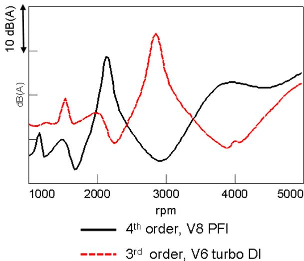
Figure 14: Comparison of dB(VINS) rear axle noise share for a V8 PFI and a V6 charged direct injected engine
