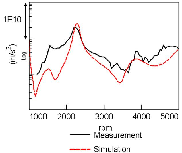
Figure 11: Axle mount vibration, active side, 4<sup>th</sup> engine order for WOT run-up in 3<sup>rd</sup> gear
