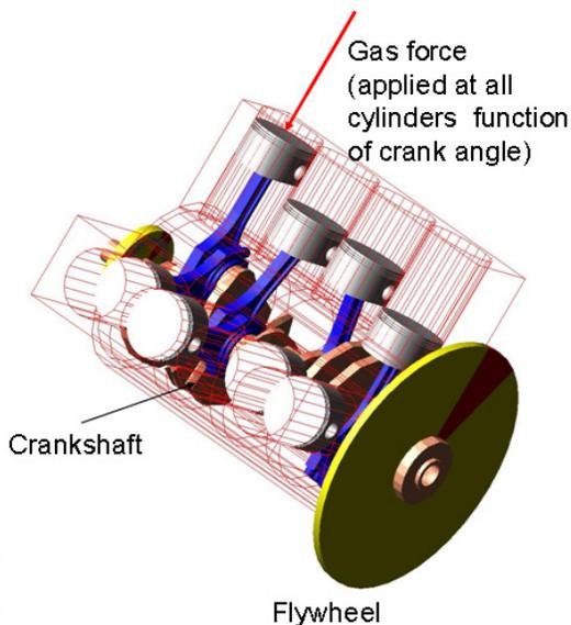
Figure 6: Virtual engine model of the V8 engine used for flywheel dynamic torque calculation
