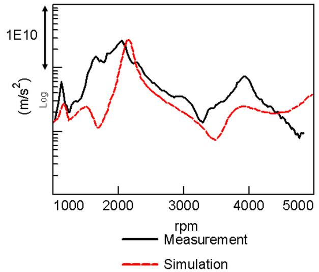
Figure 10: Axle mount vibration, active side, 4<sup>th</sup> engine order for WOT run-up in 2<sup>nd</sup> gear
