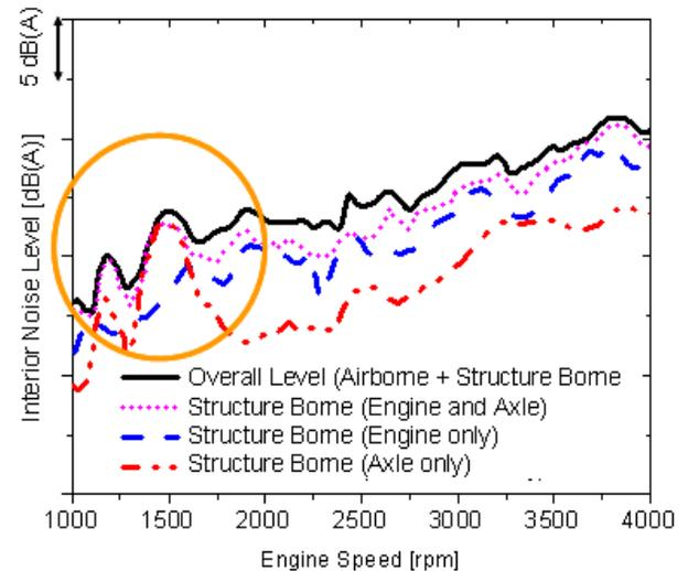
Figure 1: Noise share breakdown of a four cylinder Diesel engine propelled RWD vehicle via VINS transfer path analysis
