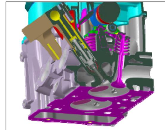
Figure 2 (above): The arrangement of the injector and spark plug in the combustion chamber
