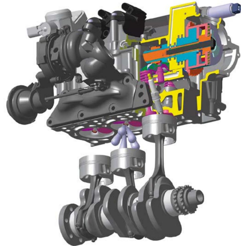
Figure 5: A small direct-injection turbocharged version of a three-cylinder gasoline powertrain equipped with a SOHC, two valves per cylinder
