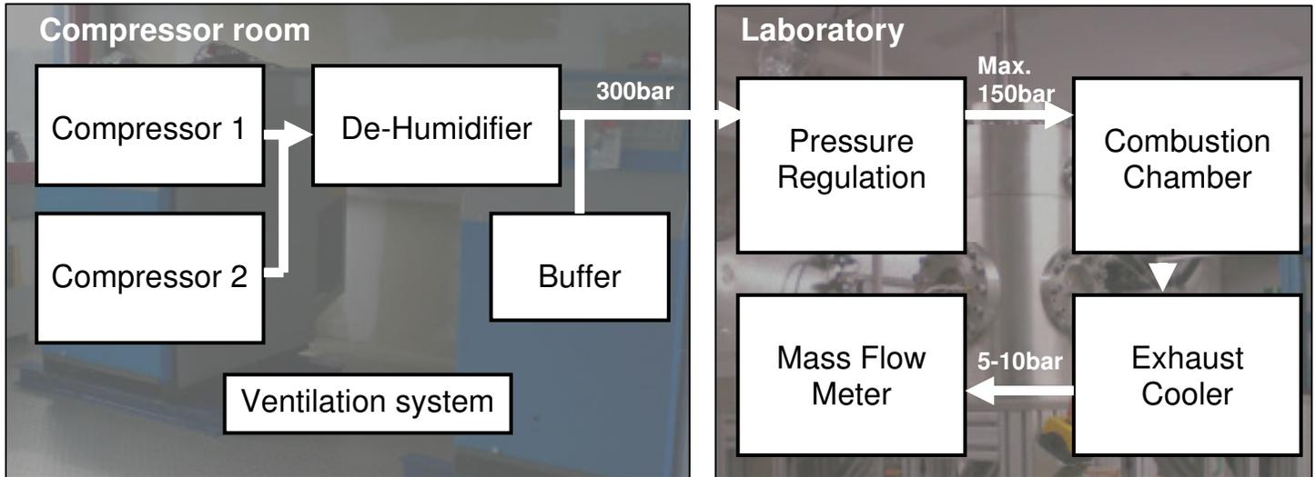
Figure 1 High-pressure chamber test bench setup
