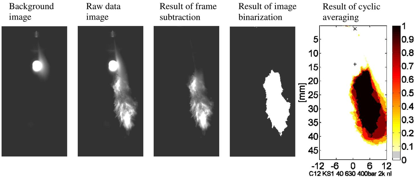
Figure 5 Raw data post-processing procedure
