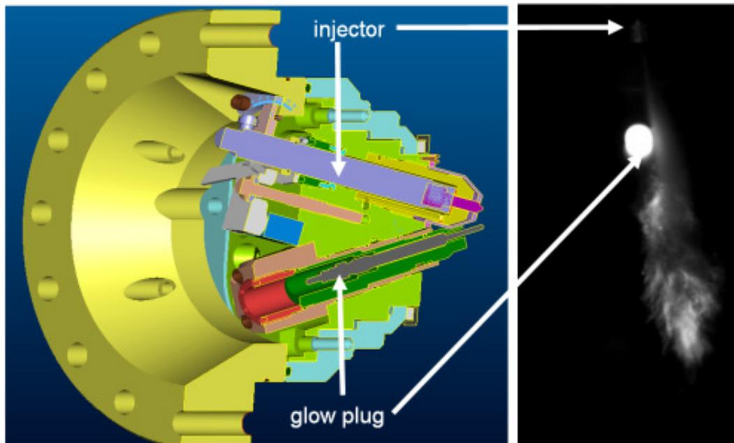
Figure 2 Customized Injector and Glow-plug holder and exemplary raw data flame radiation image in front view perspective
