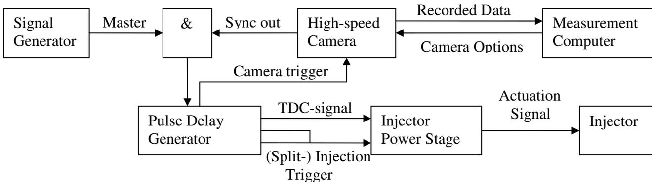
Figure 4 Triggering Scheme
