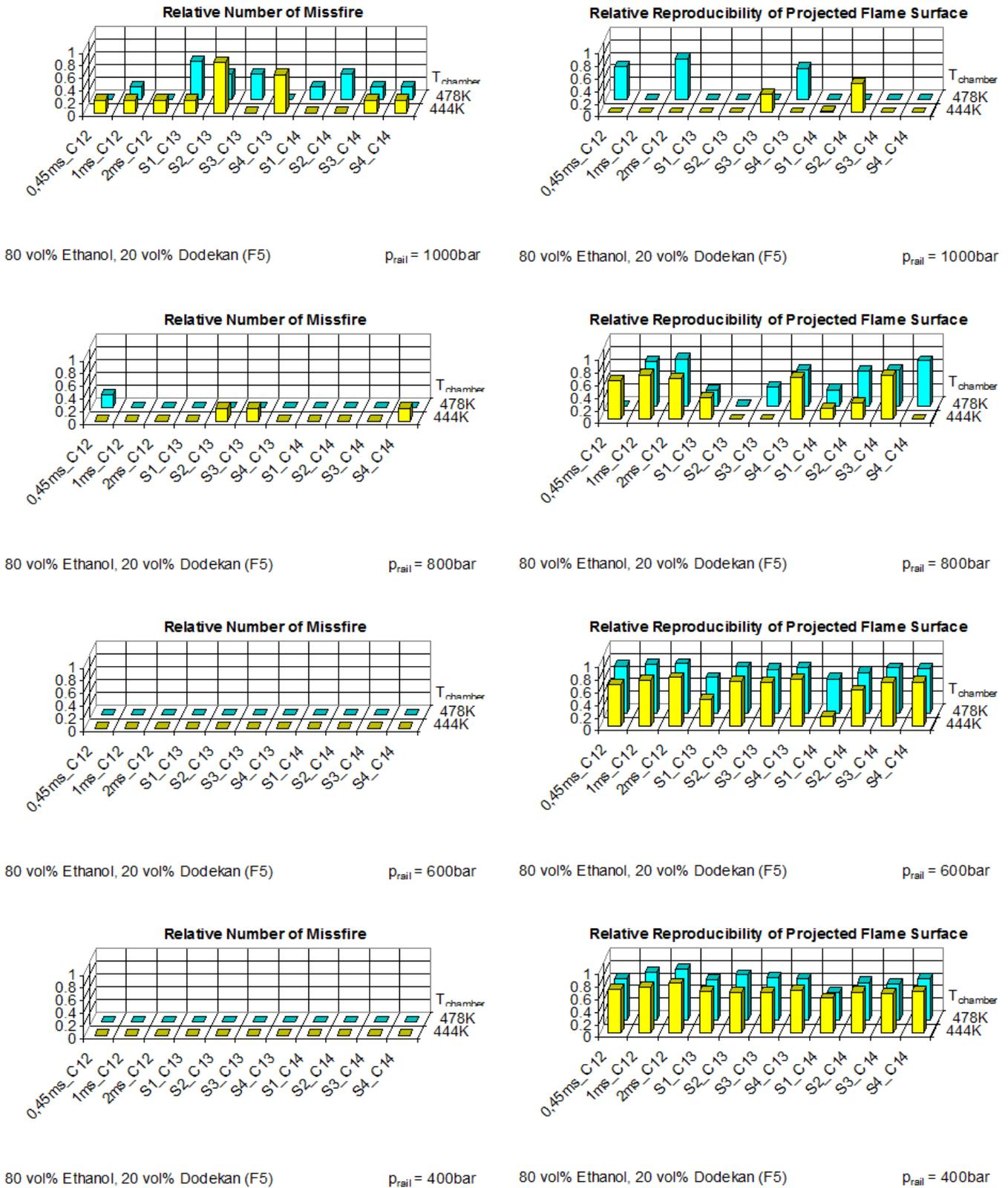
Figure 9 Statistical evaluation of glow-plug ignition stability with ethanol-dodecane mixture for varying rail-pressures
