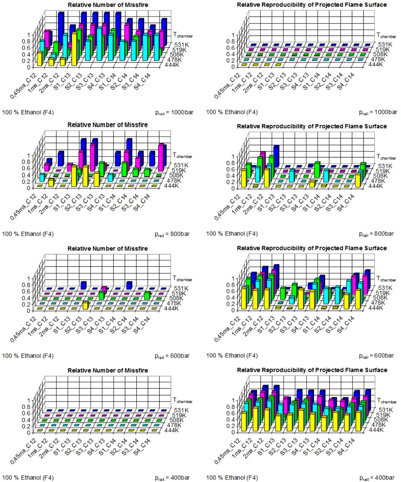
Figure 8 Statistical evaluations of ethanol glow-plug ignition stability for varying rail-pressures
