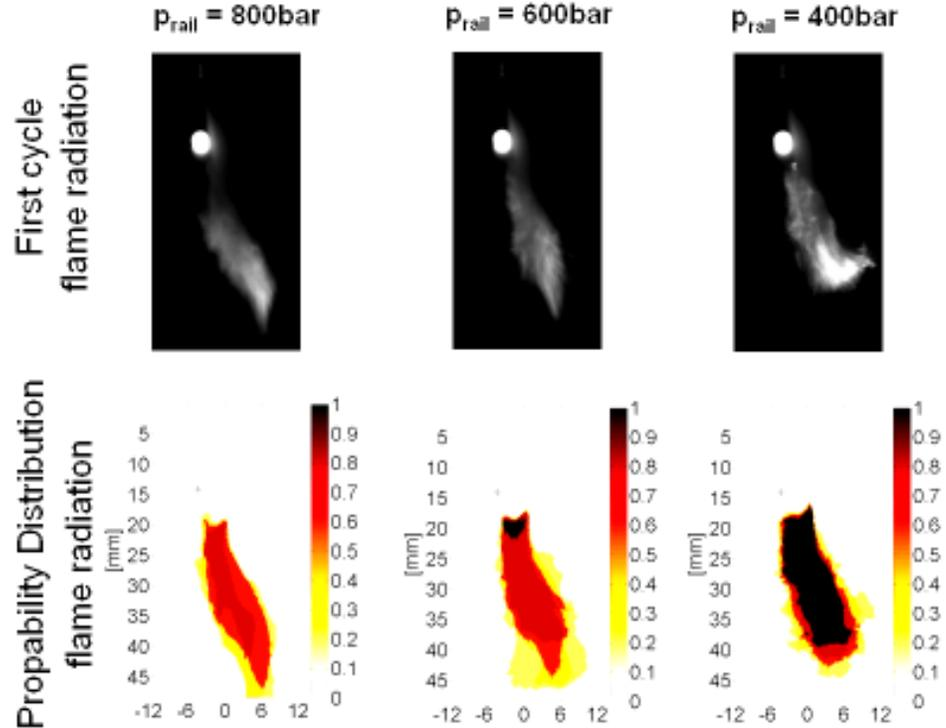
Figure 7 Effect of rail pressure on ignition behavior of ethanol
