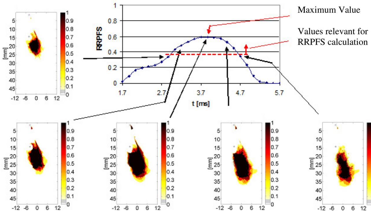
Figure 6: Procedure for the calculation of the relative reproducibility of projected flame surface
